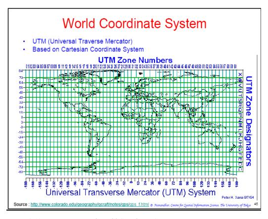
Figure 2.12: Two Dimensional World Coordinate System
