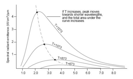
Figure 5.4: Blackbody radiation curves based on Stefan-Boltzmann's law (with temperature in k)
