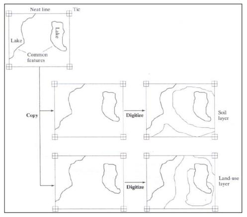
Figure 2.4: The method of using a digitizing template. Using a digitizing template eliminates the need to digitize common features on different layers and ensures perfect registration of these features when the layers are used for overlay analysis.
