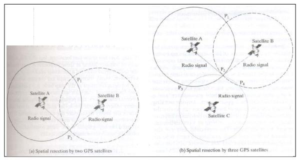
Figure 2.9: Spatial resolution by satellite ranging. Two satellites can not fix a position in space because the circles representing the satellite ranges meet at two locations, P1 and P2 as shown in (a). To fix a position, a minimum of three satellites is needed, as shown in (b). To find three-dimensional elevation, four satellites are required.
