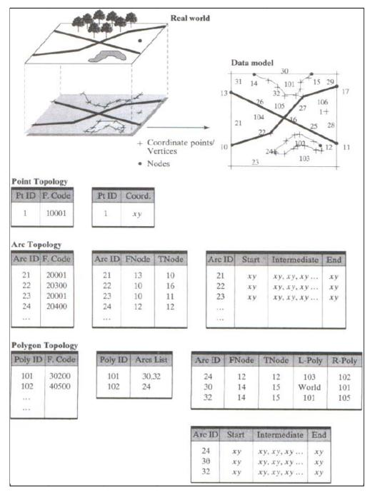
Figure 2.18: The arc-node topological data model
