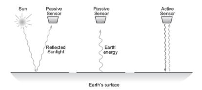
Figure 5.1: A remote sensing sensor measures reflected or emitted energy. An active sensor has its own source of energy.
