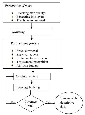
Figure 2.5: Graphical data conversion by scanning. Scanning of the map is only a small part of the whole data conversion process. Much work is needed to prepare the map before scanning and to postprocess the resulting vector data to make them useful for geographic database creation.
