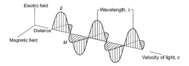
Figure 5.2: Electric (E) and magnetic (M) vectors of electromagnetic wave
