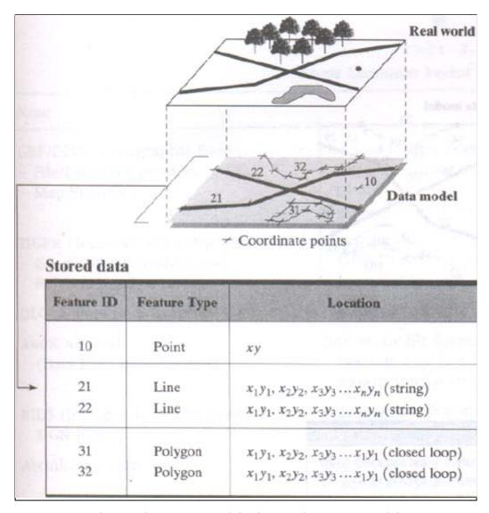
Figure 2.17: The Spaghetti Data Model. The Spaghetti Data Model stores geographic data in the form of graphical elements (point, line, and polygon), but not as graphical entities such as a lake, a wooded area, or a highway.
