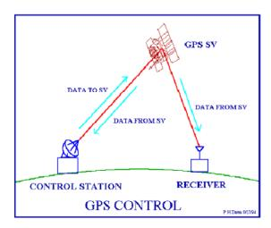
Figure 2.6: Segments of a GPS
