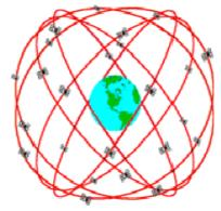
Figure 2.7: Space segment of a GPS
