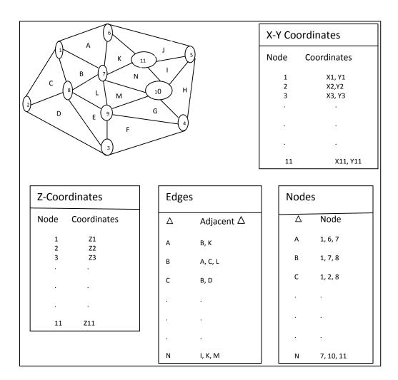
Figure 2.19: The Structure of a TIN
