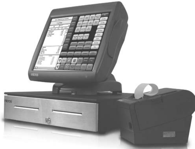
FIGURE 7-4 Electronic Cash Register: An electronic cash register typically includes a cash drawer below the server terminal. Courtesy of MICROS® Systems, Inc.
