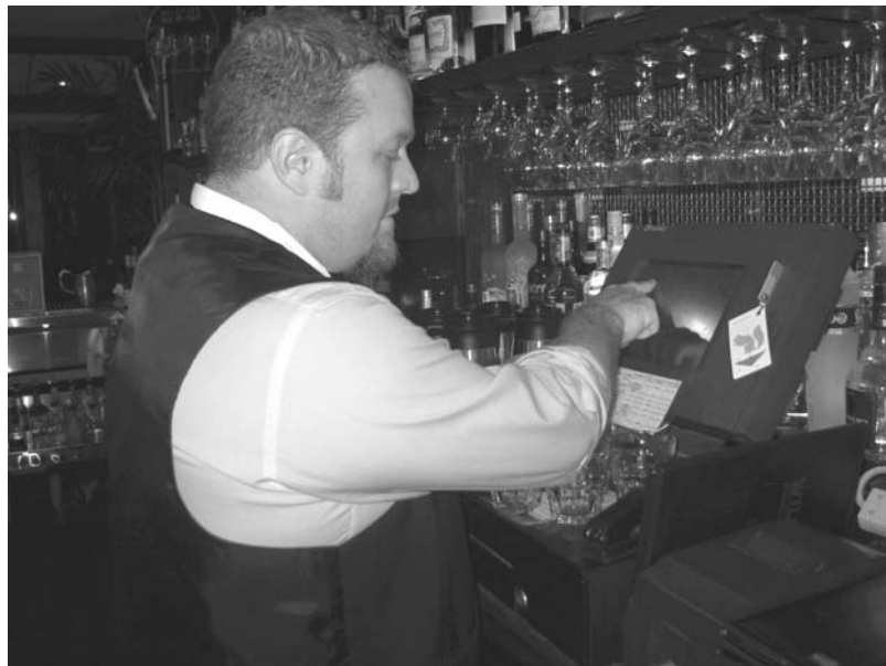
FIGURE 7-2 Server Terminal: Servers and bartenders use terminals to enter orders into the POS system. Terminals usually have a touch screen, card reader, and printer. Photo by S. Dahmer
