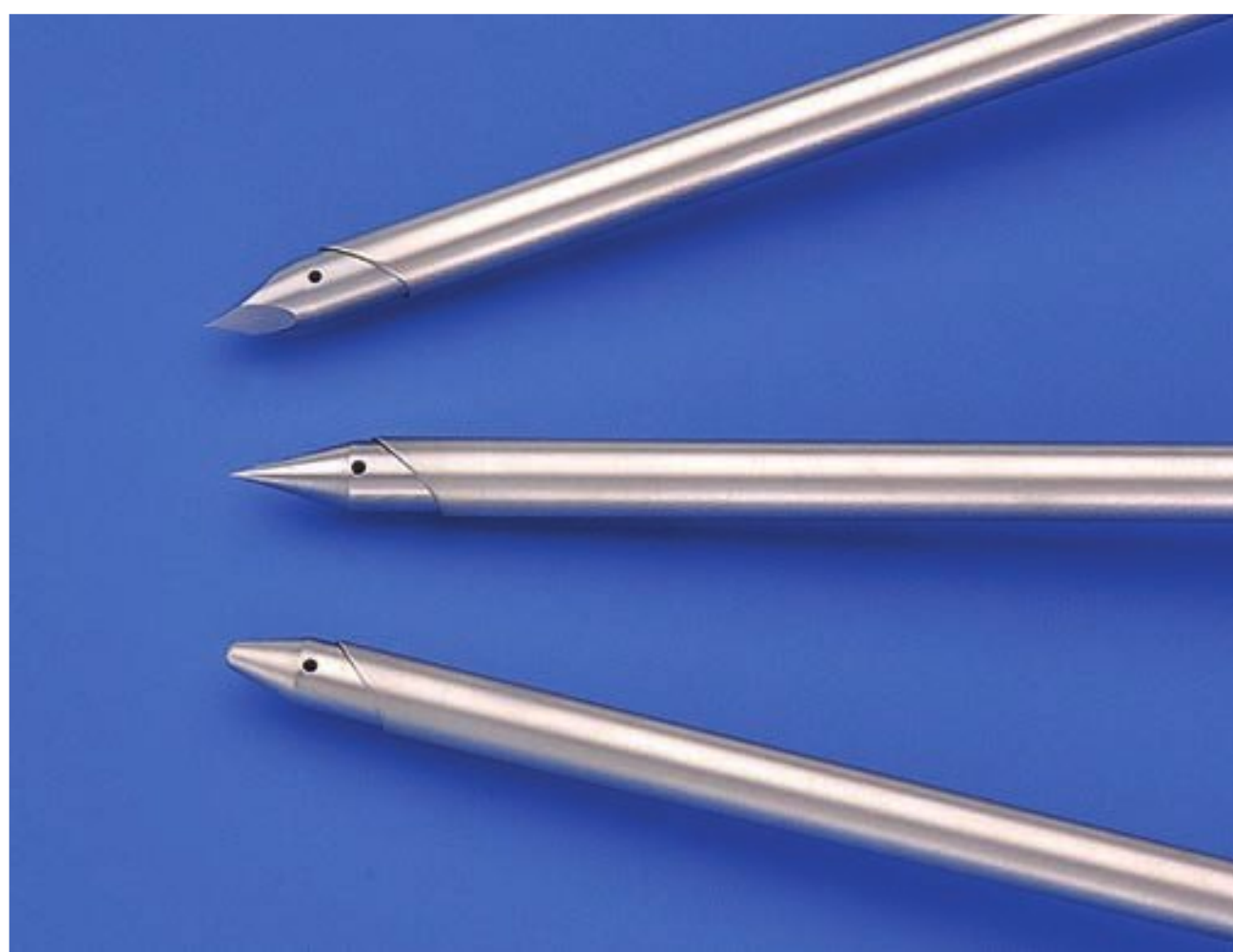
FIGURE 41-20 Trocars consist of outer cannula and inner obturator. The trocar is used to gain access to the abdomen. The obturator then is removed, and the cannula serves as a conduit through which to introduce instruments. Obturators may have a pyramidal (top), conical (middle), or blunt tip (bottom). (Reproduced with permission from Karl Storz America, Inc.)
