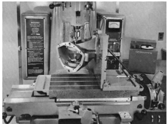
Fig. 12-27. Measuring machine setup for the measurement of the coaxiality of bearing seats bored in an automotive differential housing. A rotary recorder is used for preparing polar charts, which indicate the relative conditions of the traced bore surfaces.
