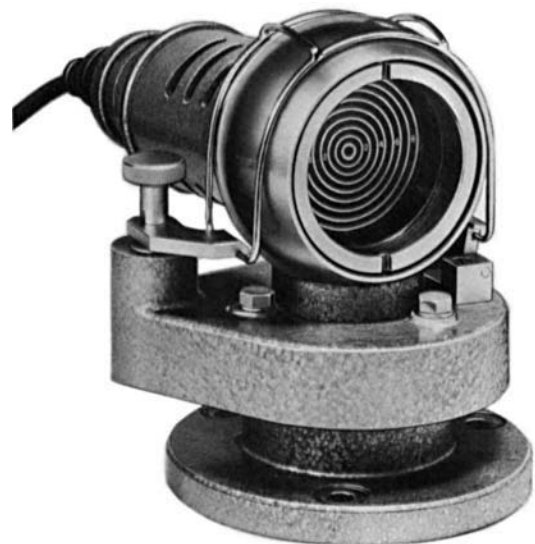
Fig. 11-13. Circular pattern target enclosed in a spherical mount and equipped with illuminator.
