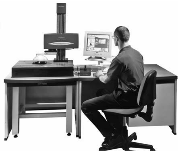
Fig. 13-3. A profile-tracing instrument capable of simultaneous assessment of form, dimension and texture in a, single traverse.
