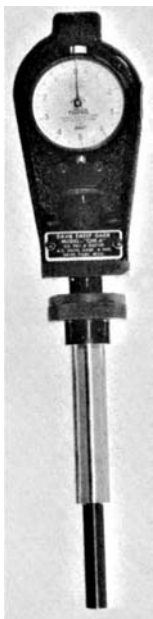
Fig. 5-53. (Left) Bore concentricity gage in one of the basic designs, with long locating body for checking a deep-lying bore.
