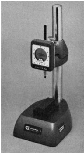
Fig. 5-37. Bench comparator stand with electronic indicator.
