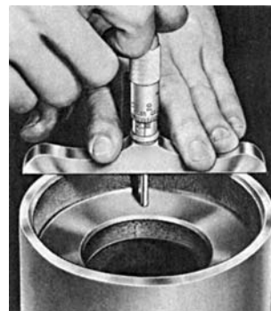
Fig. 2-34. Depth micrometer for measuring the distance of protruding features from a flat reference surface.
