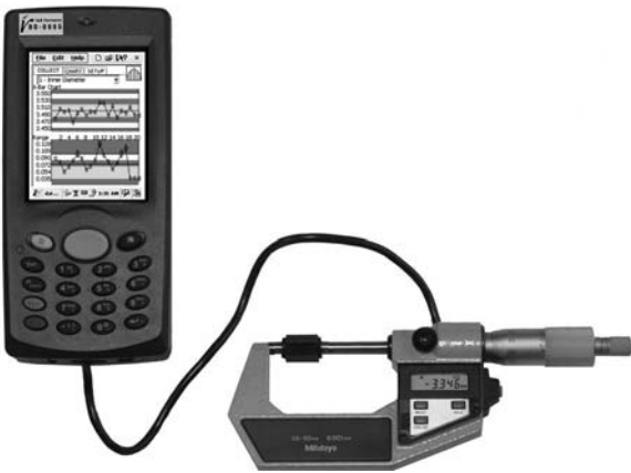
Fig. 2-40. Digital micrometer interfaced via RS-232 with the DC 9005 hand held data collection device.
