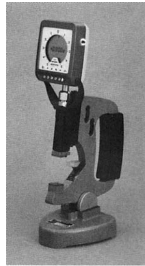
Fig. 5-31. Snap gage with electronic indicator and bench stand.
