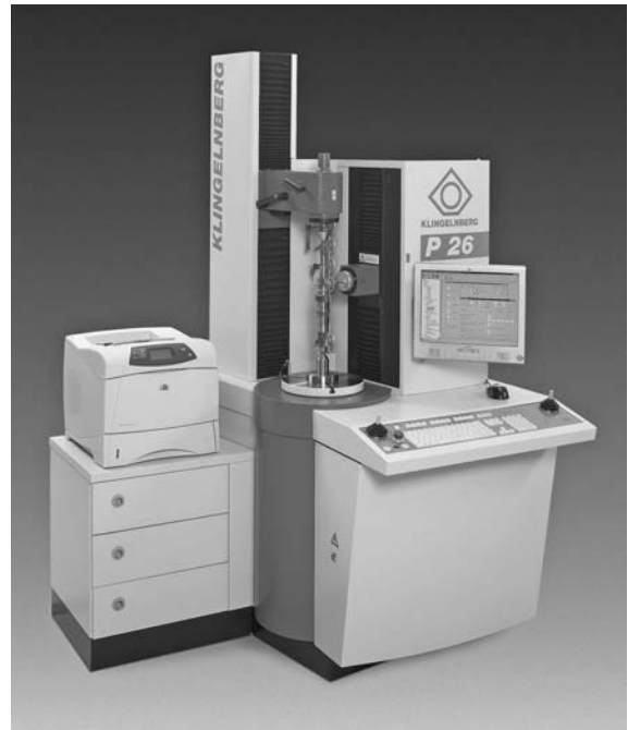
Fig. 17-25. Gear Measuring Center with combined gear element and other feature measuring capabilities.
