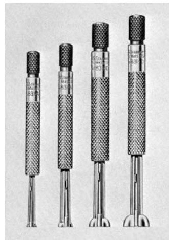
Fig. 2-29. Small hole gage for the transfer of actual bore dimension, which is then measurable with a regular outside micrometer.
