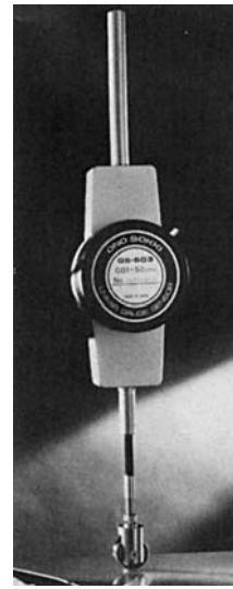
Fig. 5-21. Roller contact tip on a linear gage sensor.
