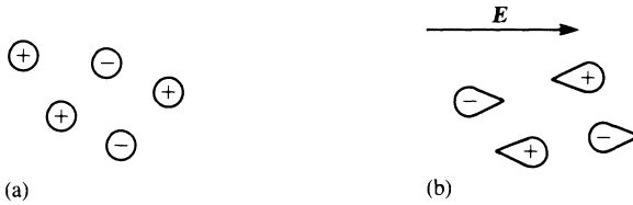
Fig. 2.5. The asymmetric effect on a solvated ion under the influence of an electric field: (a) no field; (b) with field.
