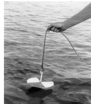
Fig 6.1. (a) A secchi disc with its cable (b) A secchi disc lowered into water body
