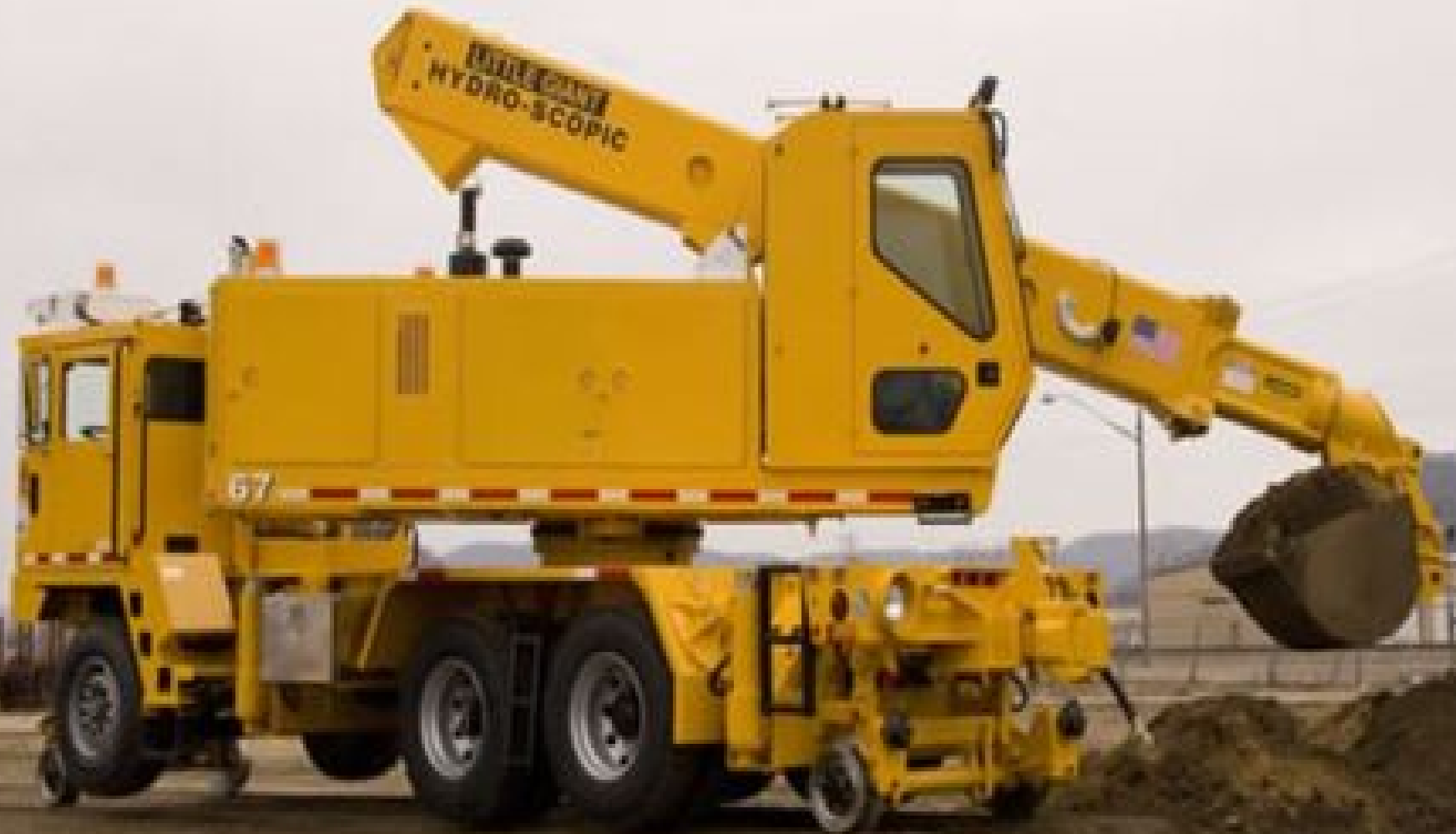
Truck mounted excavator
