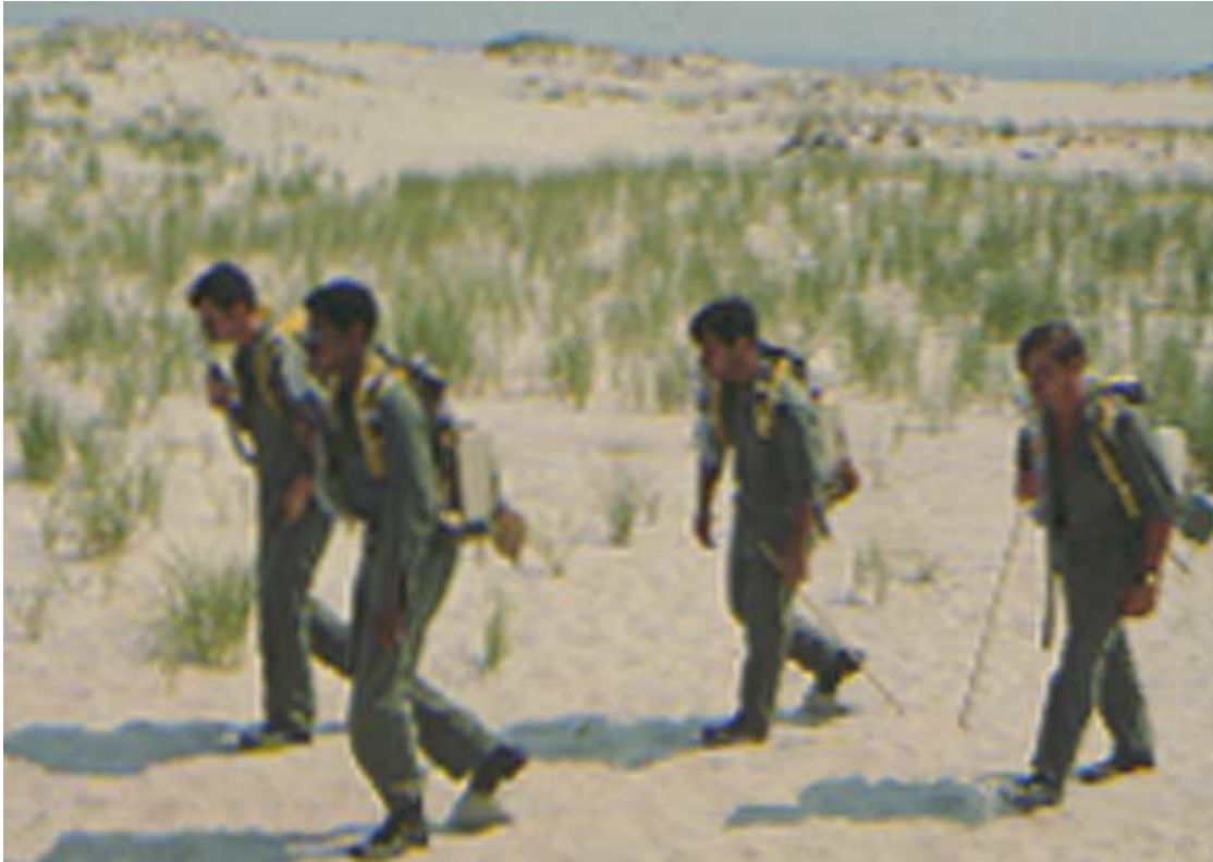
Attachment Fig. 7. The additional energy cost required to march on soft sand, found to be a multiplier (terrain coefficient) of 2.1 times the energy cost at the same march rate on a treadmill or blacktop road, is being measured in this study. 1 The military volunteer subjects are shown wearing “Max Planck” gasometers. This 7-lb gas meter measures a timed volume and the temperature of respired air, and collects an aliquot sample (0.3% of each exhalation) in the rubber bag shown hanging from the gasometer. The difference between the oxygen content of ambient air (20.93%) and the residual oxygen content subsequently measured in the sampled expired air, multiplied by the gasometer’s measured respiratory volume (L/min, corrected to standard temperature and atmospheric pressure), can be directly converted to kilocalories per minute using the factor of 4.85 kilocalories per liter of oxygen consumed. This photograph helps explain why the multiplier is so high, if one notes the amount of sand lifted with each step and recalls the finding (from an earlier study 2 ) that the energy cost of 1 pound of footwear is equivalent to that of 5 pounds carried on the back. (1) Soule RG, Goldman RF. Terrain coefficients for energy cost prediction. J Appl Physiol. 1972;32:706–708. (2) Soule RG, Goldman RF. Energy cost of loads carried on the head, hands or feet. J Appl Physiol. 1969;27:687–690.
