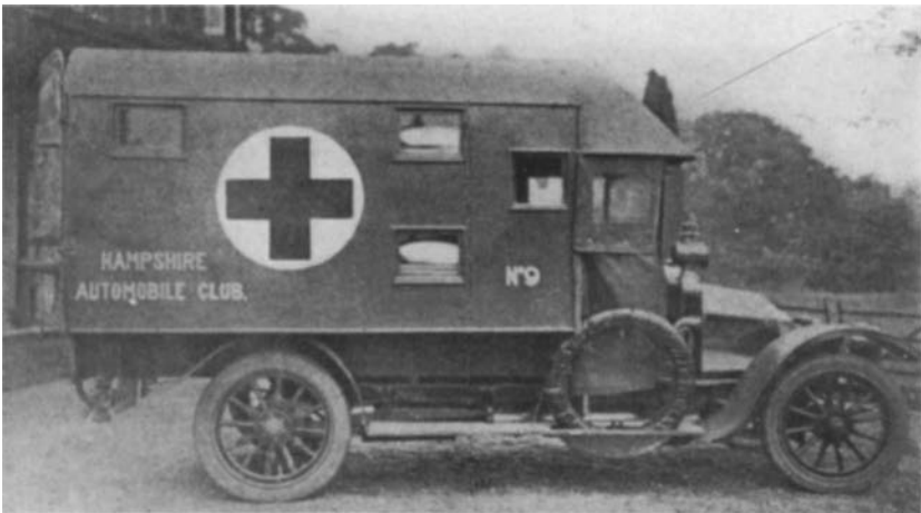
48. A Hampshire Automobile Club ambulance motorcar with three-ply wood sides, canvas top, and Hooper windows. Note protection given to the driver by the canvas cowl and side curtains. F. L. Pleadwell, "Types of Motor Ambulances Observed Abroad," Military Surgeon , XLVII (1920), opposite 332.
