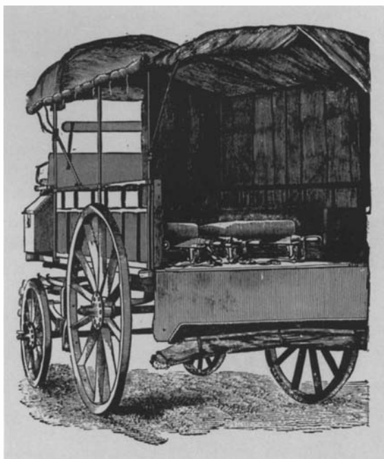
28. British army sick-transport wagon, showing the Faris stretcher on the floor of the wagon. George J. H. Evatt, Ambulance Organization, Equipment, and Transport (London: William Clowes, 1886), 72.
