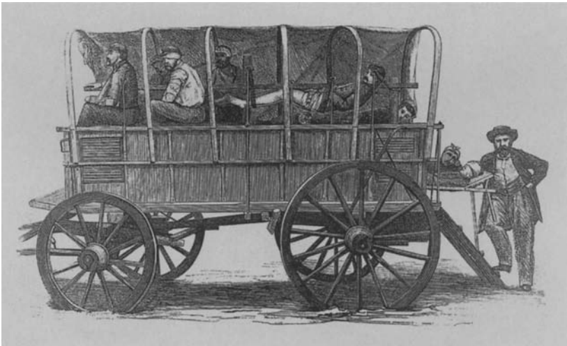
18. An army wagon fitted up as a Langer ambulance wagon. United States Government, Surgeon General's Office, The Medical and Surgical History of the War of the Rebellion , part III, vol. II, Surgical History (Washington, D.C.: Government Printing Office, 1883), 956.
