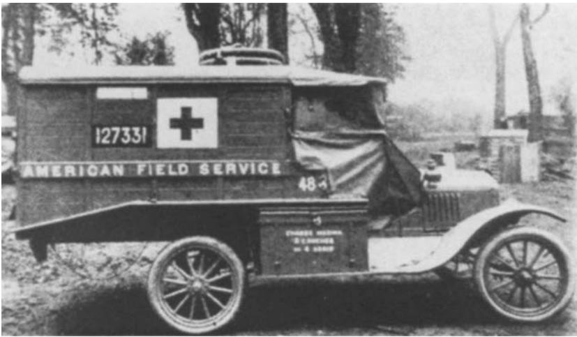
50. A Ford ambulance motorcar in the American Field Service. Note the top rack for spare tires and the side box for tools and extra gasoline. A. Piatt Andrew, "The Genesis of the American Ambulance Service with the French Army, 1915–1917," Military Surgeon , LVII (1925), opposite 363.
