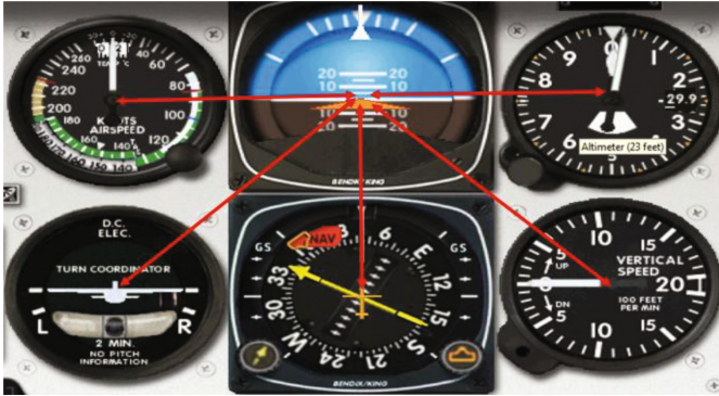
Fig. 3. Regular instrument crosscheck scenario. Instruments: Artificial Horizon (AH)– middle top position Air Speed Indicator (ASI) – left top, Altimeter (ALT) – right top, Navigation (NAV) – middle bottom row, Turn Coordinator (TC) – bottom left, Vertical Speed Indicator (VSI) – bottom right
