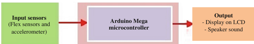
Fig. 1. Overview of the hardware components used in the sign language translator
