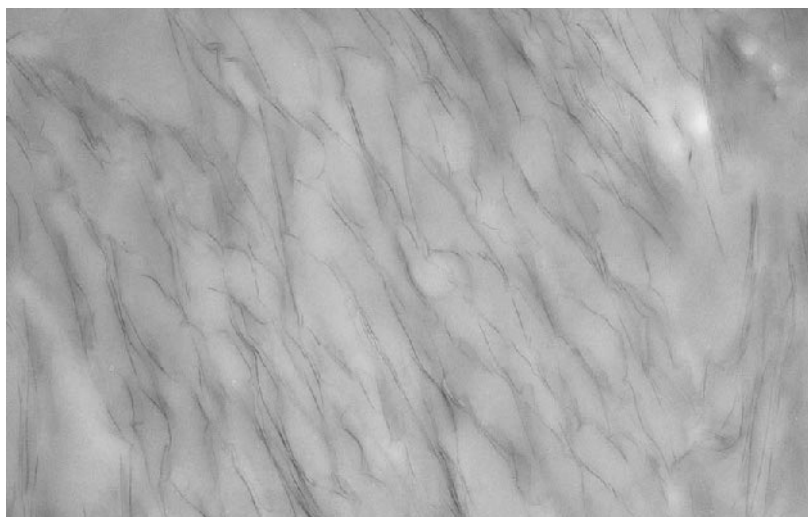
FIG. 7 TEM of polystyrene–montmorillonite nanocomposite. (From Ref. 45.)
