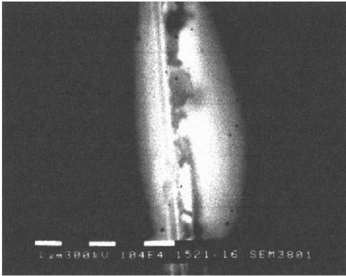
FIG. 43 SEM image of PbS–CdS–PbS superlattice.
