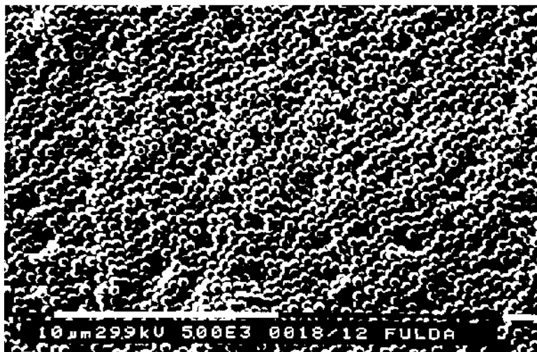
FIG. 13 SEM picture of an LB multilayer of particles 1a after transfer of five monolayers onto a glass substrate. (From Ref. 156.)
