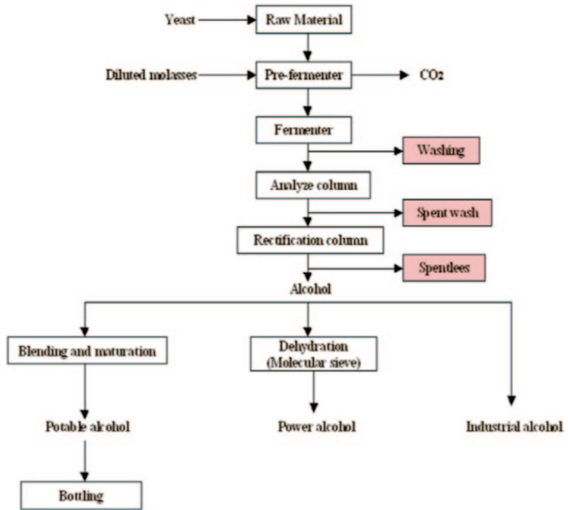
Fig. 2.1 Detailed process of alcohol production
