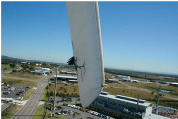
Fig. 11.14 Lightning damage at the trailing edge near the tip of a Westwind 20 kW wind turbine blade at the CSIRO Energy Centre, Newcastle. Photo courtesy of Phil May, Solartec Renewables
