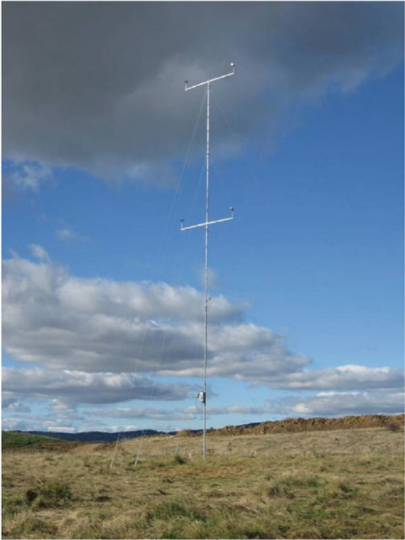
Fig. 12.2 Anemometer mast for site monitoring for a multiple small turbine installation at Orange, NSW, Australia. Photo supplied by Cyclopic Energy
