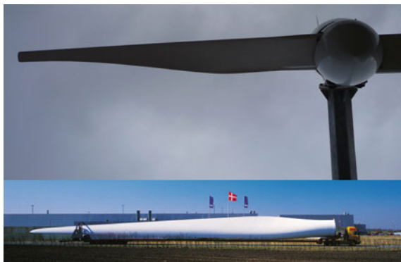
Fig. 7.6 The Aerogenesis 2.5 m long blade compared to the LM Glassfiber 61.5 m blade from www.lmwindpower.com (accessed 4 Aug 2010)
