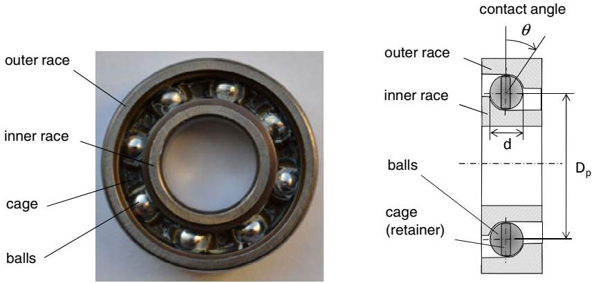
Fig. 6.35 Key elements of an angular contact ball bearing
