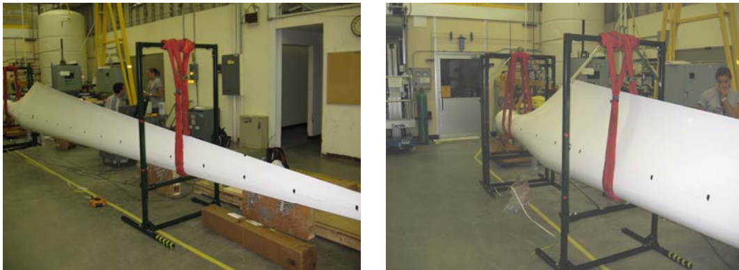
Figure 18: Tip-end frame in baseline location 6.5m from root (left) versus moving the frame to 3m from root (right)
