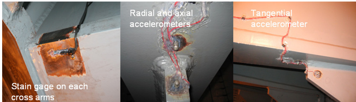
Figure 2: Rotor instrumentation
