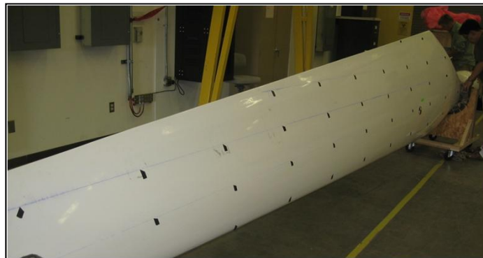
Figure 1: Measurement location grid on CX-100
