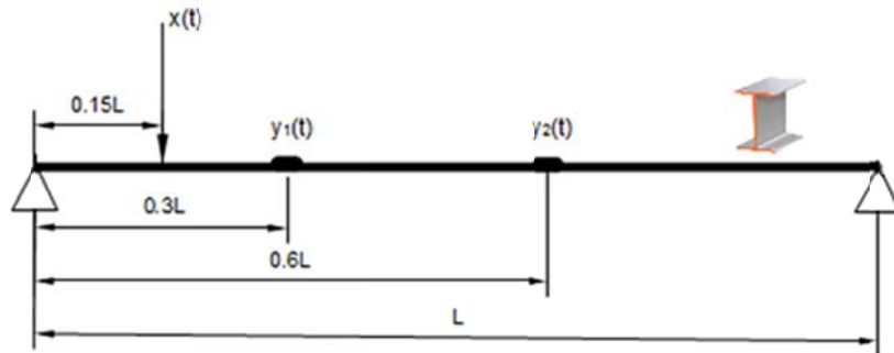
Fig. 2. Simply supported beam for model validation
