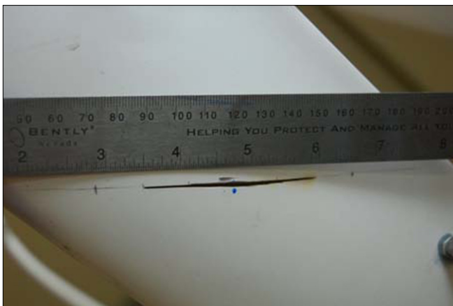
Figure 6 Surface Crack
