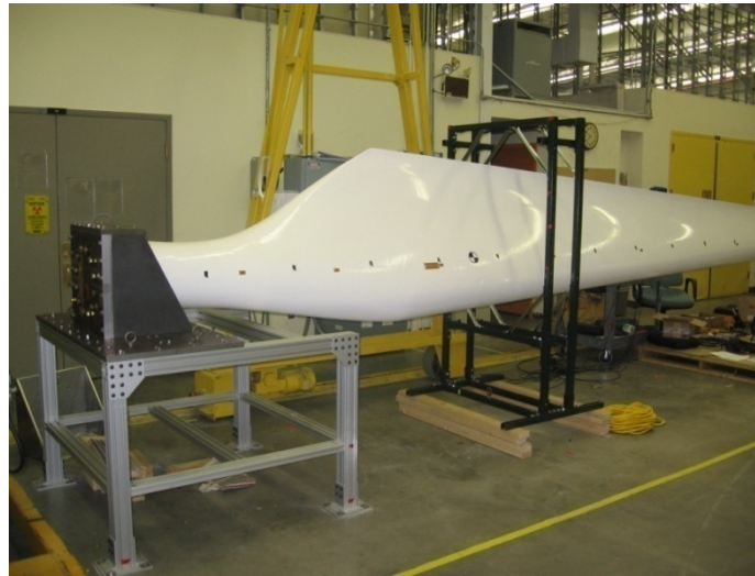
Figure 5: Blade mounted to fixture for Fixed-Free Test
