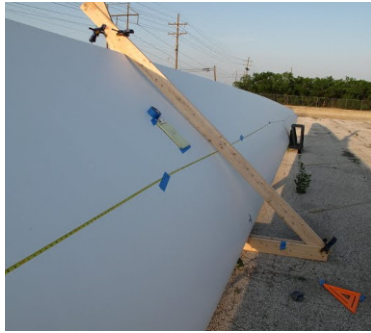
Figure 8: Measuring the Wind Turbine Blade
