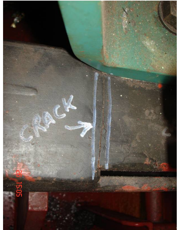
Fig. 2 Bed frame crack, starboard aft corner, transverse frame weld
