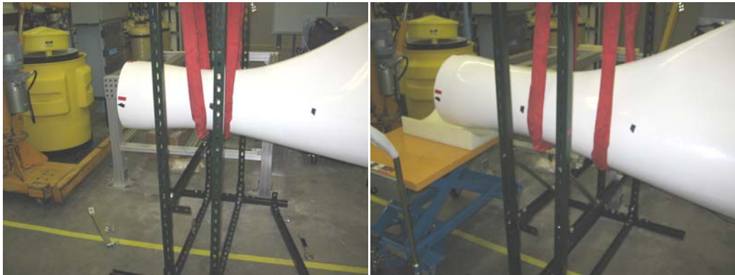
Figure 22: Root support in baseline location (left) versus moved to 0.86m from root (right)
