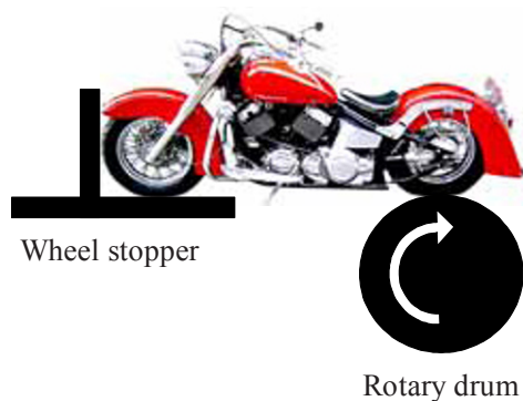
Fig.1 Actual vehicle test using chassis dynamo
