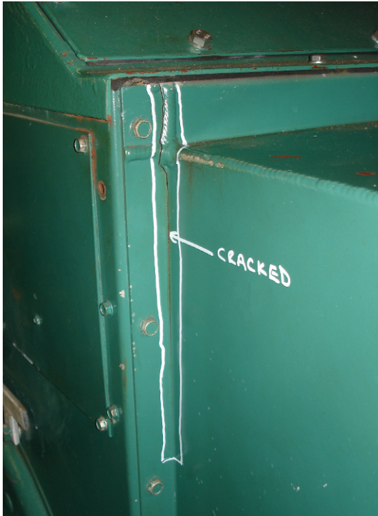
Fig. 1 Auxiliary generating set no. 1, separator housing vertical crack, port forward corner
