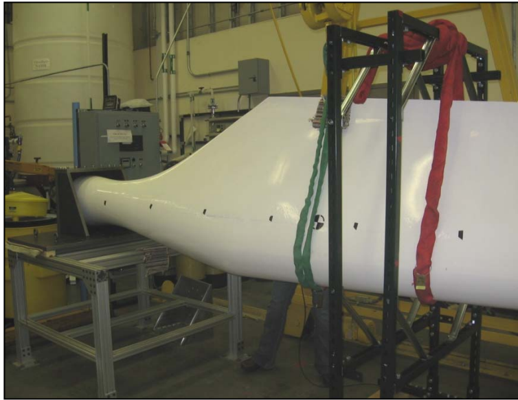
Figure 4: Free-Free Modal Test II setup with fixture bolted to blade root
