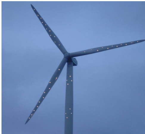
Figure 1 Distribution of the markers throughout the turbine.
