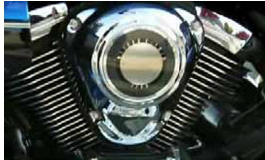
Fig.7 V type Engine
