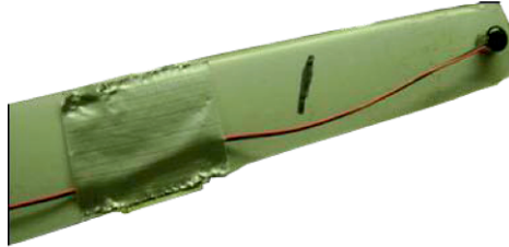
Figure 2: Accelerometer mounted to turbine blade #1.
