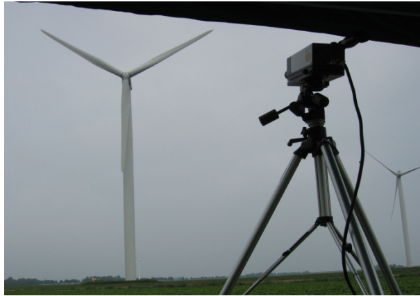
Figure 2 Laser Doppler vibrometer
