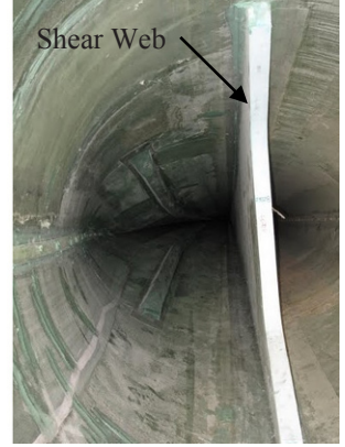
Figure 7: Suzlon Blade Interior with Shear Web
