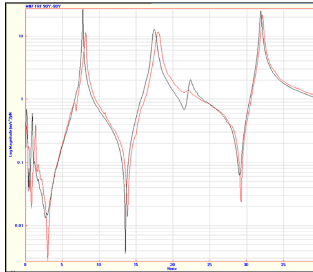
Figure 21: FRF comparison between low-pressure side contact (black) and equal side contact (red) configurations
