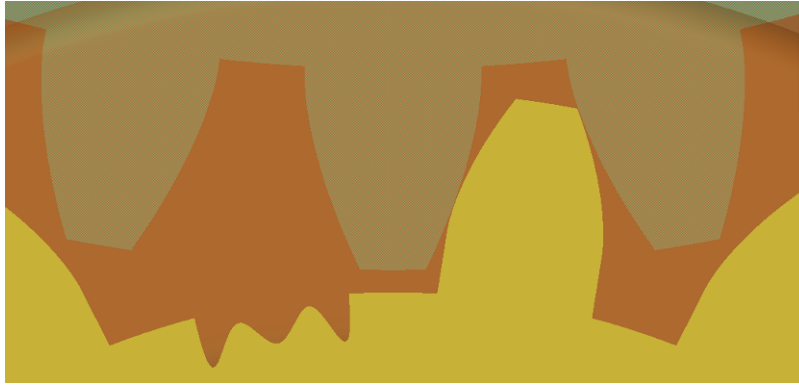
Fig.2 Chipped tooth profile
