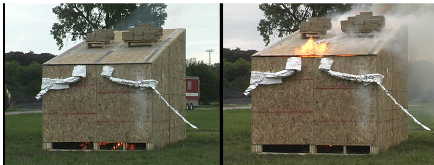
Figure 4 - WTCA burn test. Fire-sensors are shown installed and protected using aluminum wrapping.
