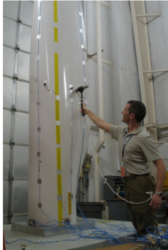
Figure 7. Impact Excitation of Blade Panel
