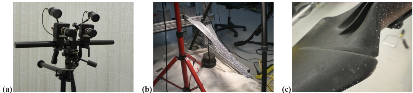
Fig. 3 Static load testing using a DIC system used to locate and track local strain concentrations. (a) Trillion DIC cameras on precision mount. (b) Example of static loading at blade mid-span. (c) Machined crack at identified strain concentration.
