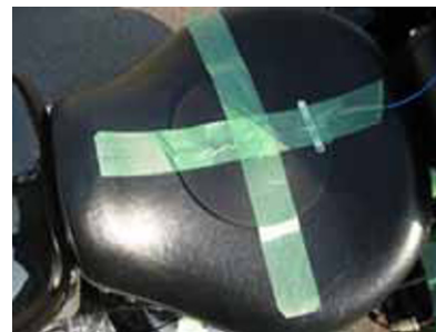
Fig.2 Appearance of sensors attached to seat
