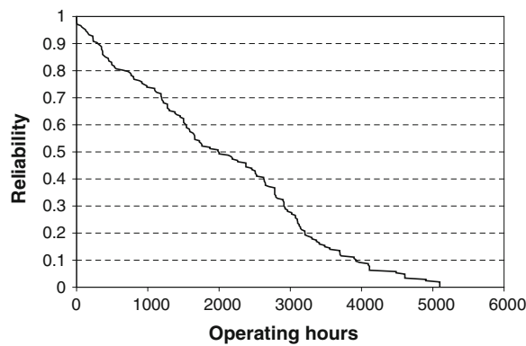
Fig. 7.11 Reliability plot of fuel injectors, based on replacement data of failed injectors
