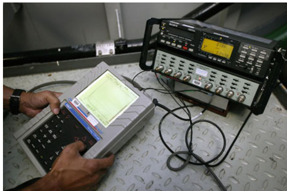
Fig. 6.14 Portable vibration analysis device
