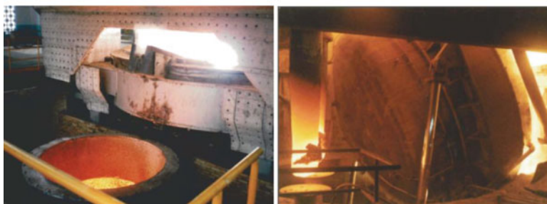
Molten BFA in mold after tilt pour.
