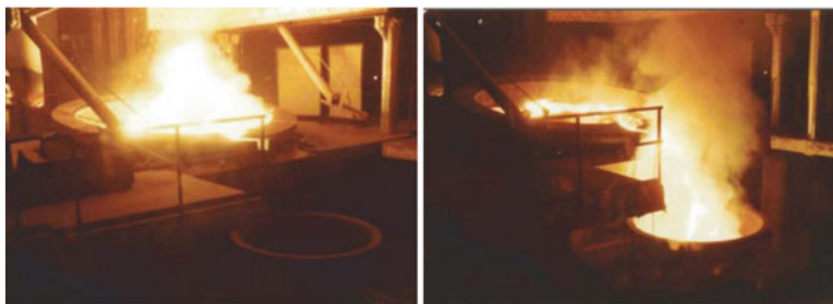
Preparing to pour, electrodes up and feed chute clear. Pouring mold (on mold car) receiving molten BFA.
