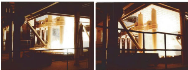
BFA pour fusion in melt position; view with level shell from work platform and pouring floor
