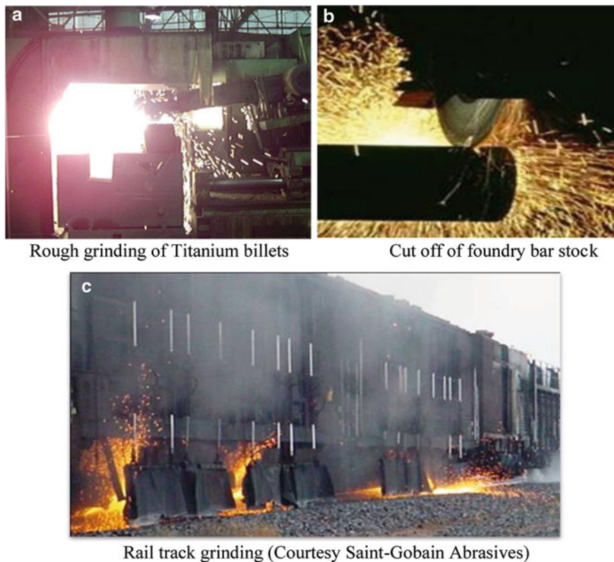
Fig. 1.31 Examples of (dry) rough grinding using grinding wheels containing coarse alumina–zirconia grain
