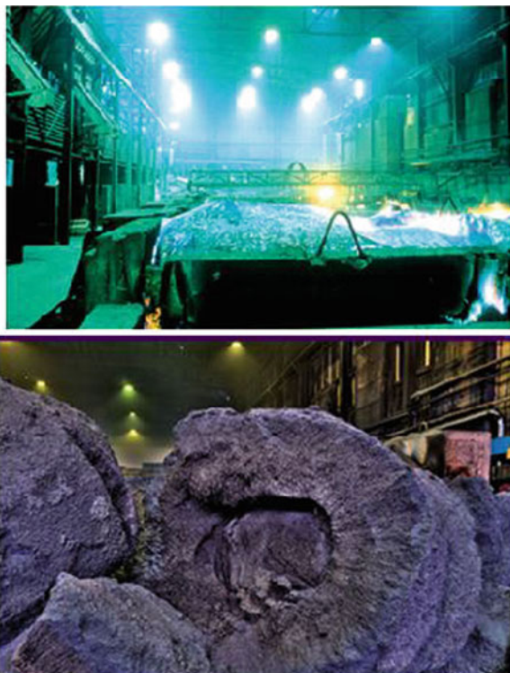
Fig. 1.17 SiC Acheson Furnaces and raw product as removed from the furnace (Courtesy Saint-Gobain)
