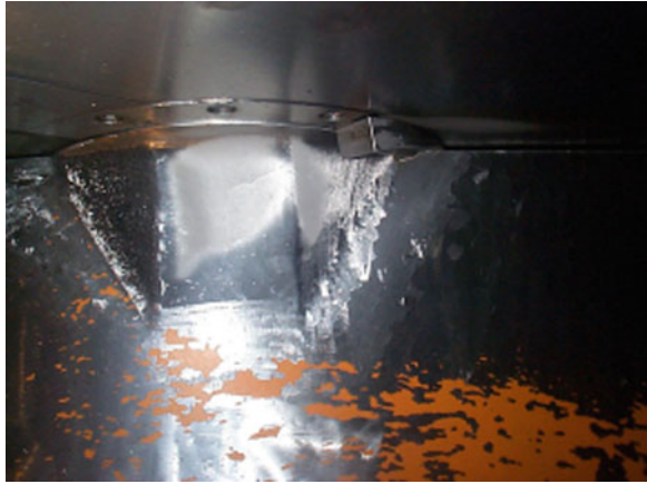
Fig. 5.4 Cavitation damage on wicket gate at stem junction
