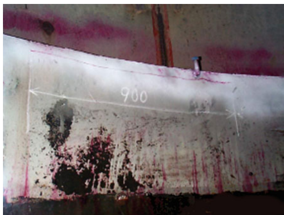
Fig. 2.12 Crack at junction of discharge ring to draft tube liner
