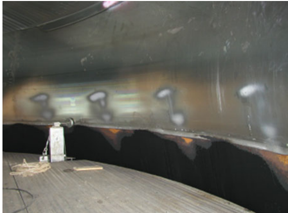
Fig. 5.5 Cavitation damage on discharge ring due to interaction between wicket gate wake and blade tip gap
