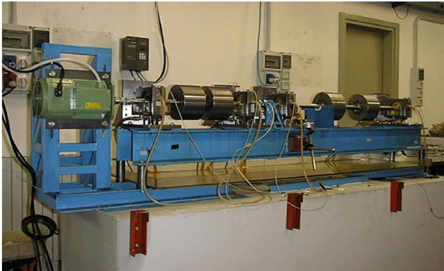
Fig. 6.3. 2-shafts and 4-oil film bearings MODIAROT test-rig.
