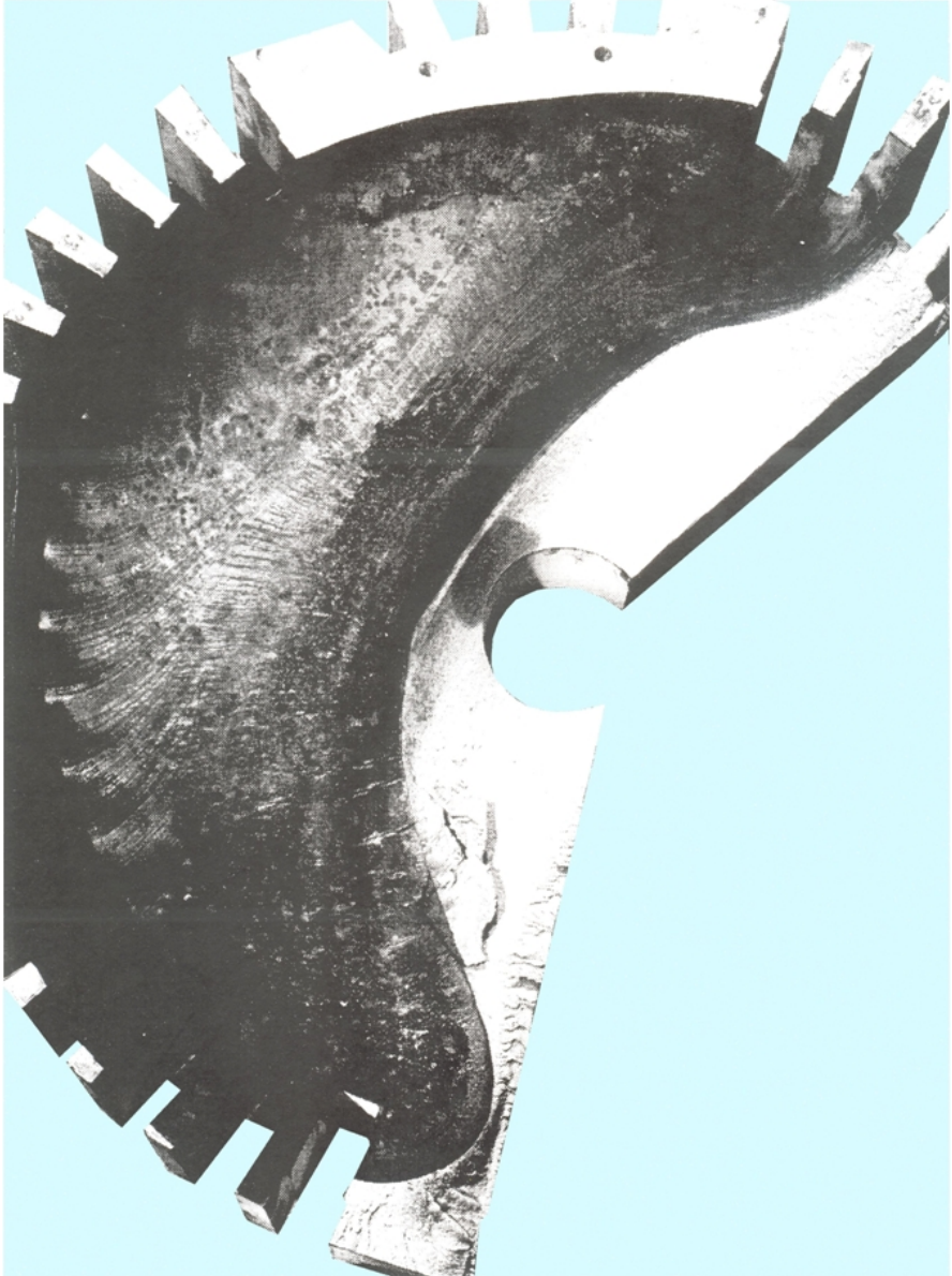
Fig. 2.15. Crack depth with respect to rotor section.
