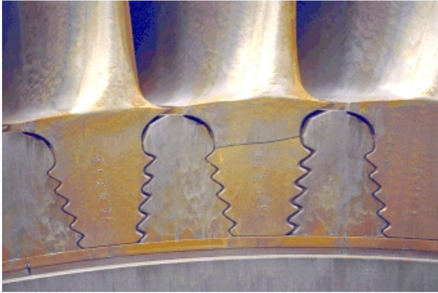
Fig. 1.2. Crack developed in the blade root of a steam turbine (Courtesy of Dr. Carlo Stoisser, Generation, Thermal Engineering Dept. EDF – Électricité de France).
