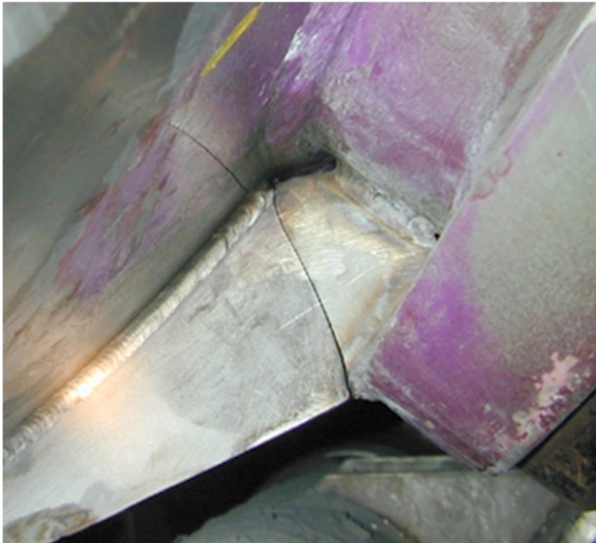
Fig. 1.1. Crack developed in the stiffening plate of a generator (Courtesy of Dr. Carlo Stoisser, Generation, Thermal Engineering Dept. EDF – Électricité de France).
