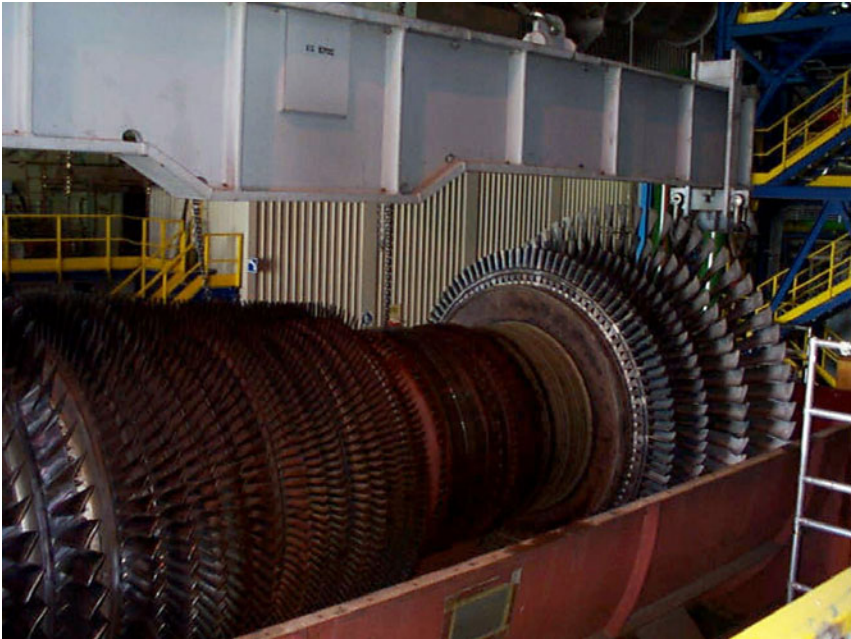
Fig. 8.13. Compressor and turbine of a gas turbo generator with case open. Due to the presence of the working fluid it is generally not possible to have a measuring plane inside the case.
