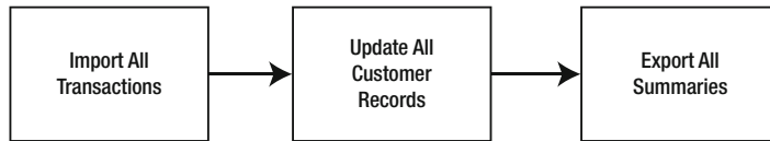
Figure 4-2. Flow of data through a batch process
