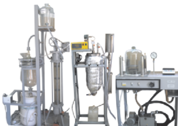
Fig. 2.1.1. Pilot installation for TA production.
