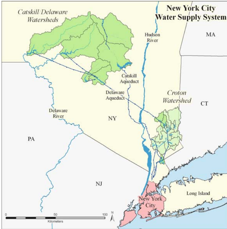
Fig. 24.1 The Catskill, Delaware, and Croton System catchments of the New York City Water Supply
