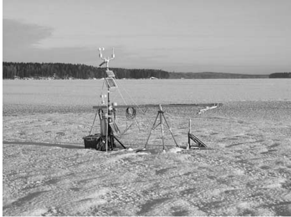
Fig. 5.1 The automatic station used to acquire data on the development of ice in Pääjärvi, the lake site used to test the new ice model
