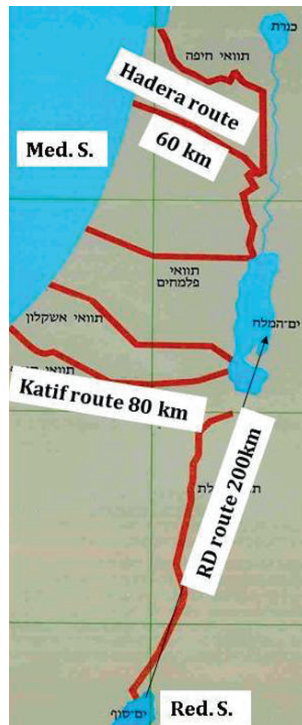
Figure 13. The six alternative routes for a seawater conduit that have been investigated by Ne'eman Committee (Source: Raz, 1993)
