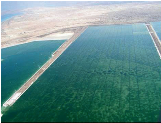
Figure 8. The potash companies' solar evaporation ponds (Photograph courtesy of Gundi Shachal of Kibbutz Ein Gedi)
