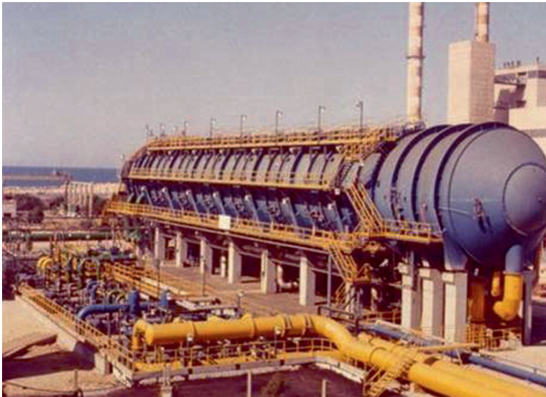
Figure 6. An LT-MED seawater desalination plant prototype (Photograph courtesy of IDE Technologies Ltd.)
