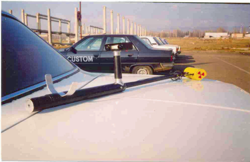
Figure 3. Developed by us the neutron portable search device with ^{252}\text{Cf} source
