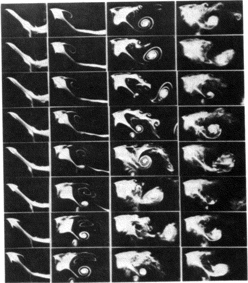
Vortex Splitting in Constant Accelerating Flow past a NACA 0015 Airfoil at angle of attack \alpha = 40^\circ and Reynolds Number Re = 1000 . Courtesy P. Freymuth, Prog Aerospace Sci. 22 (1985). Numerical solution of partial differential equations can now simulate such vortex dynamics. See pp. 346–347.
