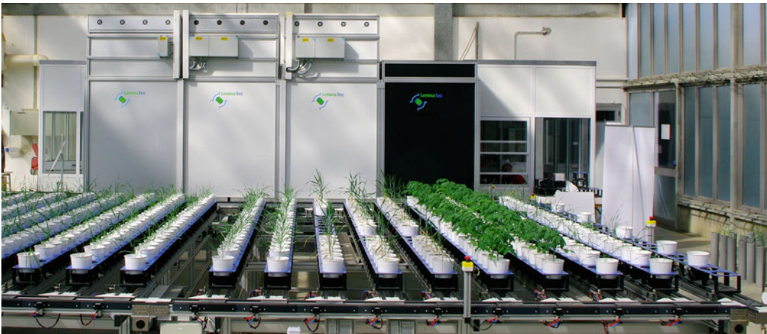
Fig. 1 The Scanalyzer 3D (LemnaTec GmbH) phenomics imaging system at the Metapontum Agrobios Research Center. The foreground of the image contains the plant storage system with conveyor belts that carry the plants to the imaging chamber. In the background and in the direction of travel for the plants (i.e. from right to left ) are: in black, the soil NIR, next the fluorescence, then the visible light, and finally the plant NIR imaging chambers
