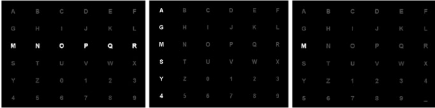
Fig. 12 Left, mid panels: row/column speller. Right panel: single character speller
