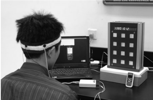
Fig. 8 Application of the SSVEP-based BCI for making a phone call. The system consists of two-lead EEG recording hardware, an LED visual stimulator, and a laptop
