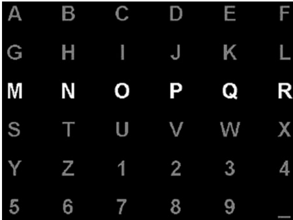
Fig. 10 The stimulus matrix shown on a computer monitor for a P300 BCI speller. One row or one column of the matrix flashes successively in a random order
