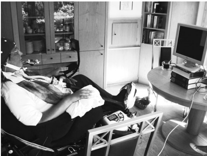
Fig. 2 Dr. Ursula Broermann sitting in front of the BCI computer screen (supported by encyclopaedias). On the left one can see the patient in a wheelchair with the electrode cap on. The wheelchair is slightly tilted to the back to stabilize the head into the chair. This way, the head does not need to be supported with a head band, which would influence the signal quality. Beside the wheelchair, in the middle of the picture, one can see the artificial ventilation machine. The amplifier is sitting on a chair besides the patient (no visible in this picture)
