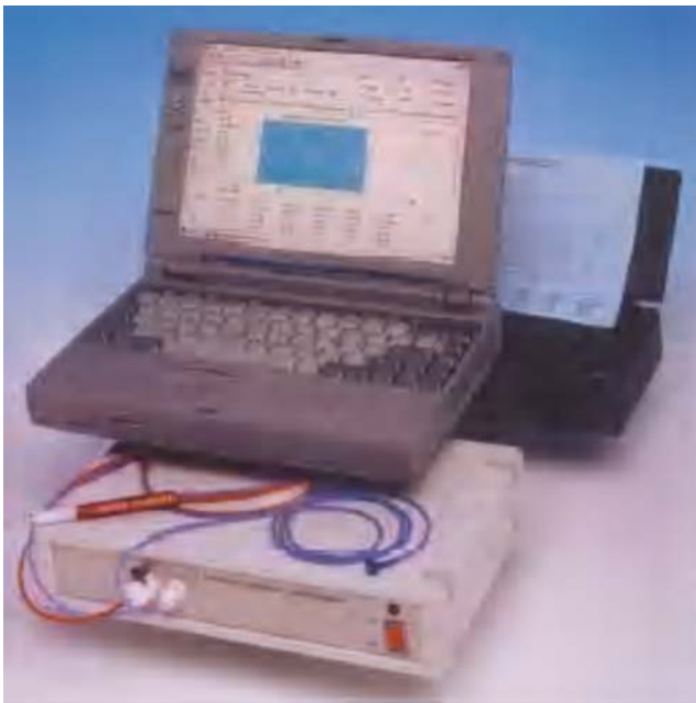
FIGURE 13.4. The Langham pneumatic digitized tonometer: The output of the pressure sensor is fed into a personal computer and is analyzed using specifically designed software on a Windows-based program. The number of complete IOP pulses is chosen by highlighting them for immediate analysis (see Fig. 13.3) and the results are printed as a hard copy. The Langham tonometer box also has a vacuum system, controlled by the computer, for modifying the IOP. This vacuum system is connected to a scleral suction cup that is applied to the sclera to induce a predetermined IOP. In addition, the cup is used to increase the IOP for measurement of aqueous humor dynamics and the ocular arterial pressure
