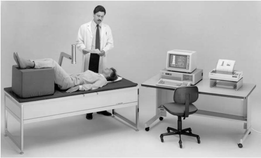
Fig. 1-8. An early Lunar DP3 dual-photon absorptiometer. This device utilized ^{153}\text{Gd} to generate photon energy. Photo courtesy of GE Healthcare, Madison, WI.
