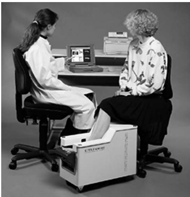
Fig. 15-34. The Osteometer DTU-one Ultrasure ® . A peripheral quantitative ultrasound device. Shown here in use. Photograph courtesy of Osteometer MediTech, Hawthorne, CA.
