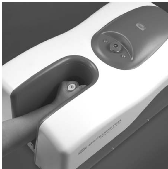
Fig. 15-21. The Osteometer DEXACARE ® G4. A peripheral dual-energy X-ray absorptiometer. The forearm is placed into the well on the top of the machine. Photograph courtesy of Osteometer MediTech, Hawthorne, CA.
