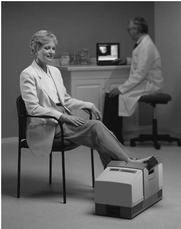
Fig. 15-25. The Lunar PIXI ® . A peripheral dual-energy X-ray absorptiometer shown here in the configuration used to measure bone density in the calcaneus. The device can be re-configured and used to measure bone density in the forearm. Photograph courtesy of GE Healthcare, Madison, WI.
