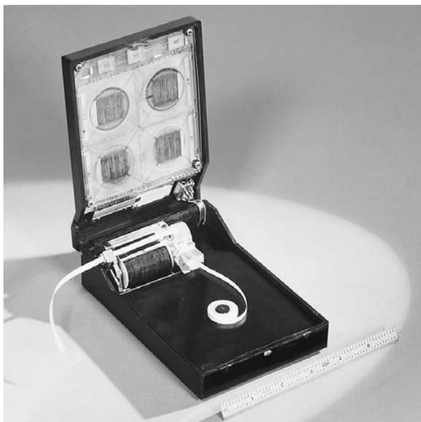
View of the inside of the first miniature calculator, invented at Texas Instruments in 1967. CORBIS/SYGMA.
