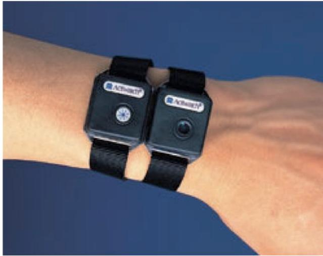
**Figure 4.2** Picture of an actigraph (Used with permission. Courtesy of Mini Mitter® Co. Inc)
