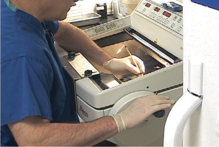
Fig. 4.5 Illustrates proper body position. Sitting with arms draped as comfortable as possible to achieve correct hand position. The arrow shows that there is still a degree of hyperextension at my wrist in this model cryostat. There are limitations to what positions are achievable in any given cryostat design. The deeper the cryostat stage below the front of the cryostat the more difficult it will be to achieve a comfortable position. Adjusting the stage to a higher position may relieve some hand stress
