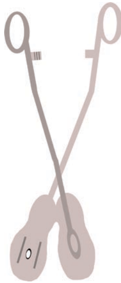
Fig. 8.10 Miami Special clamp. One of the two spatula shaped end portions is designed with a hole and grooves to accept a variety of common cryostat chucks and hold them in position ( left side of illustration). The right side spatula holds the tissue in position atop the chuck. The chuck is clamped into fixed position like a common hemostat allowing the sandwiched tissue and chuck to be dipped into liquid nitrogen to complete the freezing process
