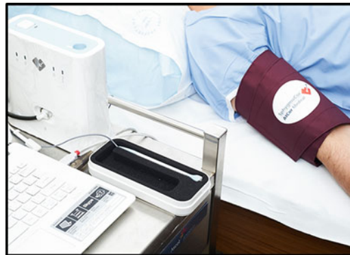
Fig. 8 PWV and PWA procedures: SphygmoCor XCEL brachial cuff used to measure systolic and diastolic pressures
