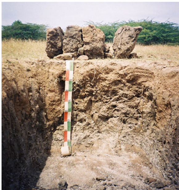
Fig. 18.5 Degraded sodic soils with columnar structure, Nalukottai series in S.No. 77, Arasani village, Sivagangai block
