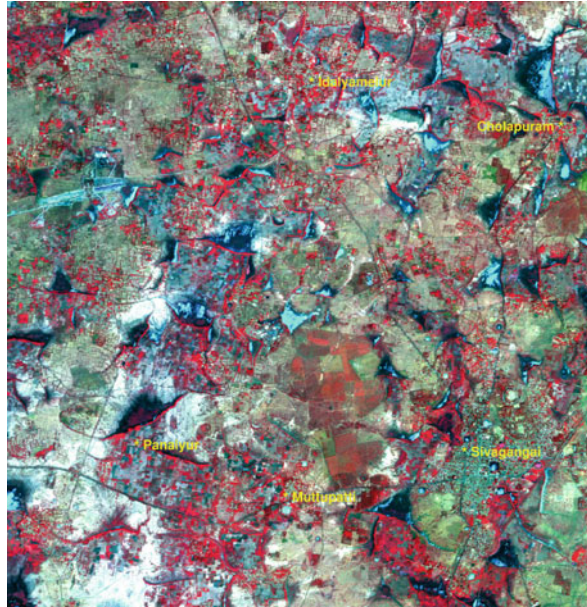
Fig. 18.6 Salt affected soils seen as a white tone on the FCC imagery from Resourcesat LISS-IV/P6, Panaiyur area, Sivagangai block, Sivagangai district, Tamil Nadu
