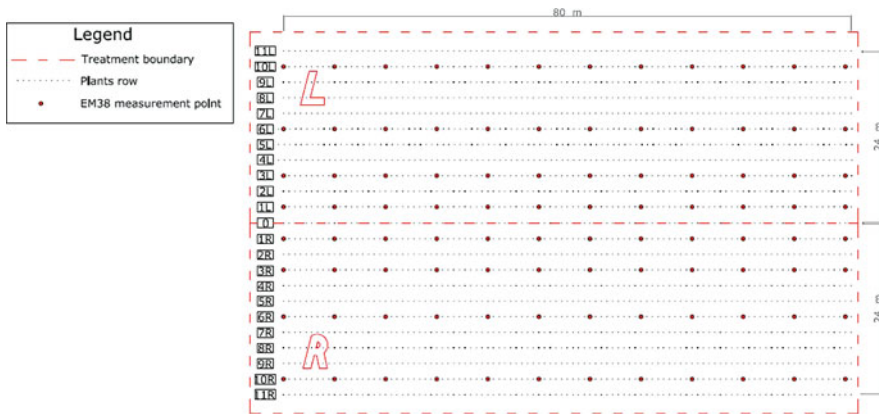
Fig. 35.2 Left (L) and Right (R) treatments at the Foraci farm, plants rows and EM-38 measurement points
