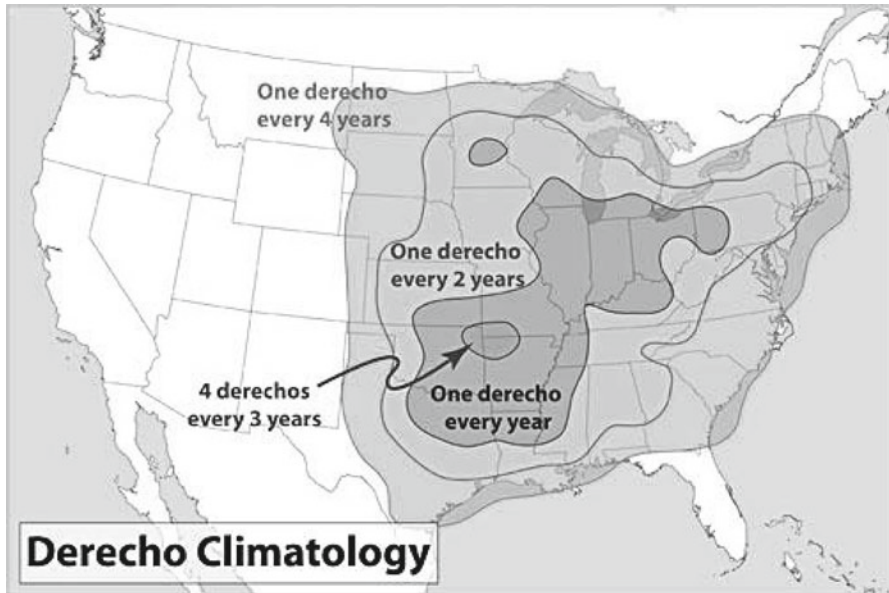
Fig. 5.10 Geographic distribution of frequency of derechos in the eastern USA (From NOAA Storm Prediction Center, 'About Derechos' FAQ website, accessed 10 December, 2014)
