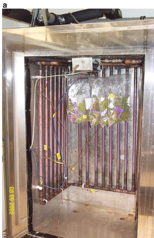
Fig. 5.2 (a) A freezing chamber used in measuring the frost hardiness of tree seedlings or organs. The plastic bags contain shoots of Pinus sylvestris seedlings. To prevent root damage caused by the freezing, the shoots have been detached from the root system. (b) Visible damage caused to Pinus sylvestris seedlings by artificial freezing. To prevent wilting, the cut ends of the detached shoots are kept in water (The unpublished photographs were provided by Risto Rikala)
