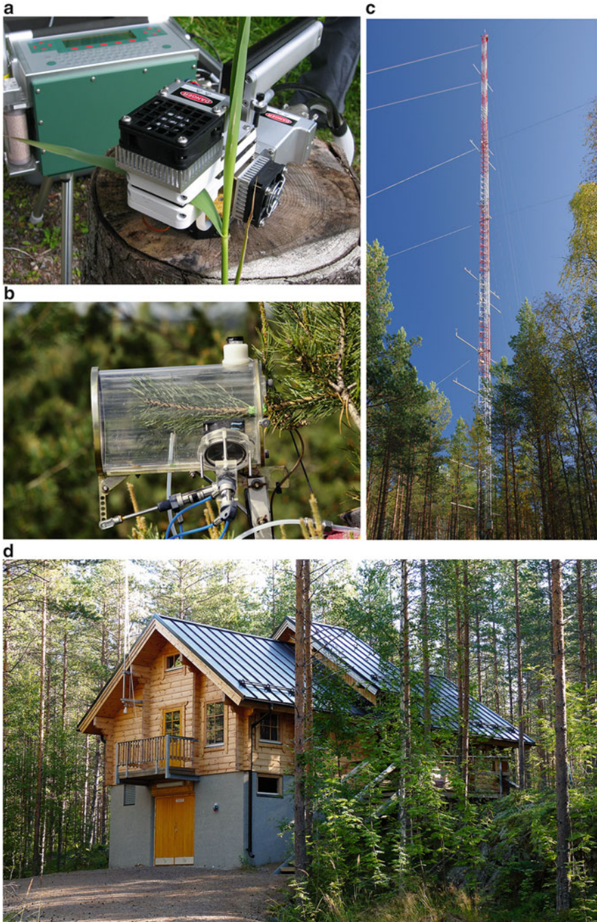
Fig. 4.1 Equipment and facilities used in studies of the CO 2 exchange of trees and other plants. (a) Portable photosynthesis-measuring system LI-6400, shown with the measuring cuvette at the front. (b) A shoot from a Pinus sylvestris tree growing in natural conditions, placed in a measuring
