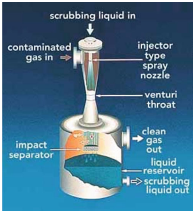
Fig. 11 Schematic of a cocurrent venturi scrubbing system
