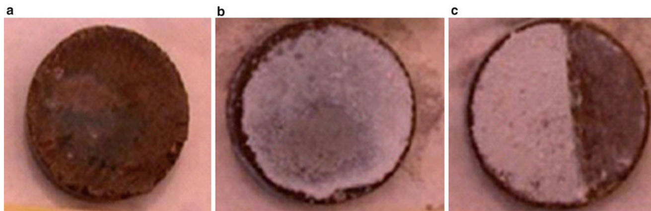
Fig. 1 Acidification and destruction of concrete specimens by the strain Acidithiobacillus (Thiobacillus) concretivorus NCIMB 8345 in 6 months. (a) The blank specimen of concrete; (b) the inoculated specimen covered with biogenic crust of gypsum; (c) the inoculated specimen where part of the crust has been removed to show its thickness
