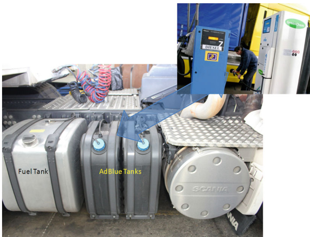
Fig. 12 Implementation of urea-SCR for LD vehicles would require the installation of a urea distribution network
