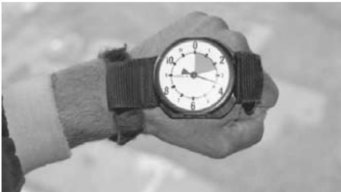
Figure 5.11 Many skydivers wear an altimeter on their wrist. This altimeter shows that the jumper is at 3500 feet.
