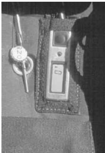
Figure 5.9 A Cypres AAD may be installed on your reserve parachute.
