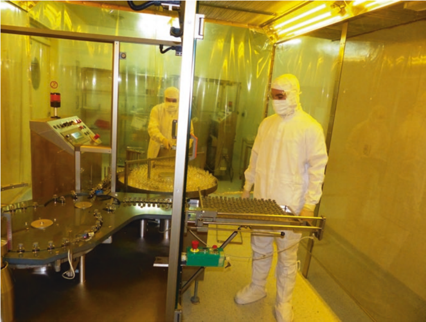
Fig. 16 Filling and stopping of Candid #1 vaccine in ten-dose vials
