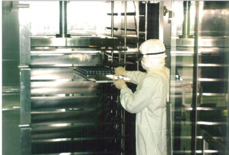
Fig. 17 Translation of pre-stoppered vials into the freeze dryer chamber before the freeze dry process
