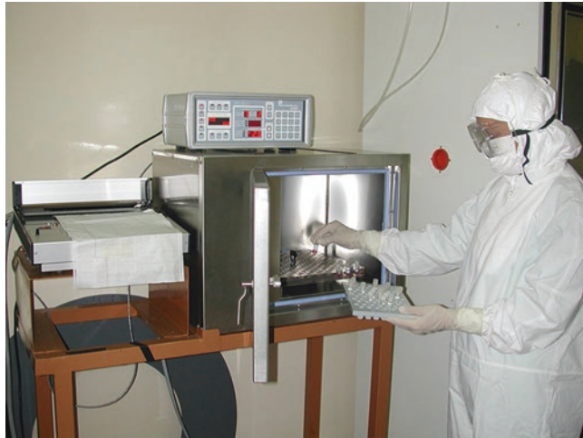
Fig. 10 Freezing of cell ampoules using a progressive cooling rate equipment to end in storage at -196^{\circ}\text{C}
