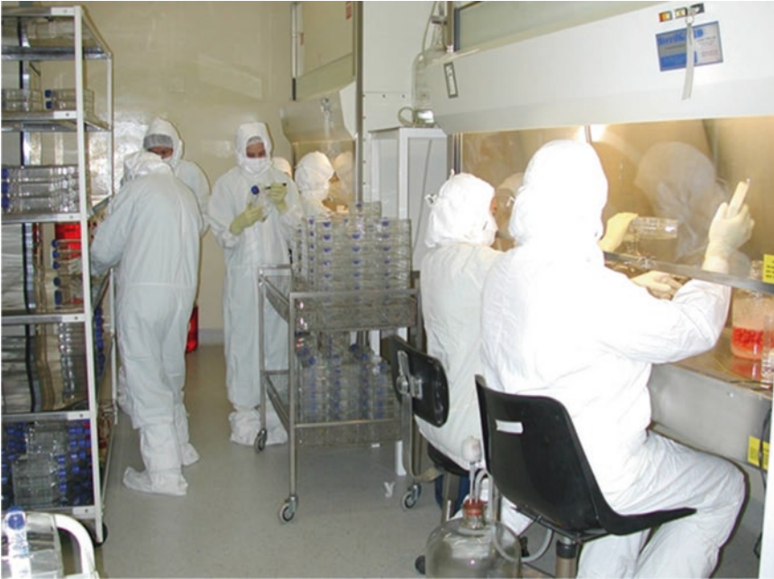
Fig. 14 Cell culture washing and viral inoculation during the manufacture of Candid #1 bulk vaccine
