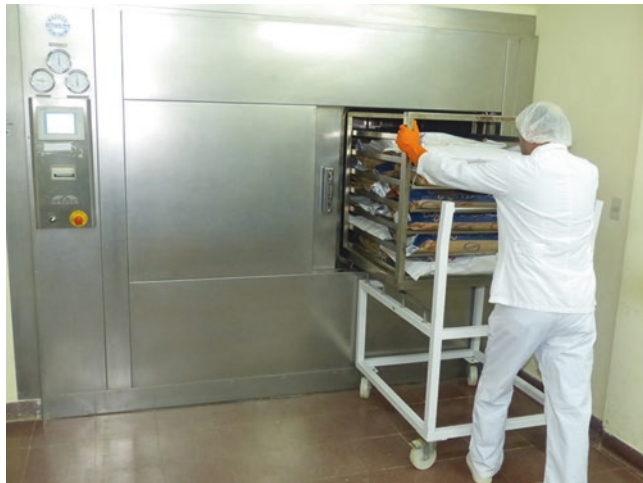
Fig. 7 View of the foremost autoclave to treat food, beverage, and bedding before entering the SPF area of the mouse-breeding colony
