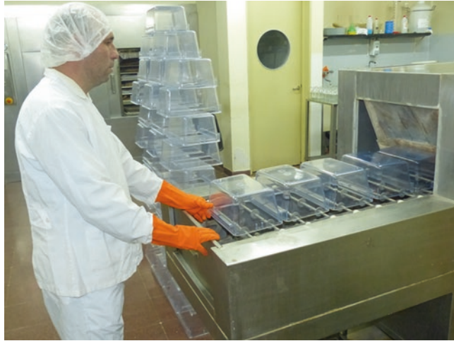
Fig. 6 Automatic washing of cages in the ancillary area of the SPF mouse breeding colony
