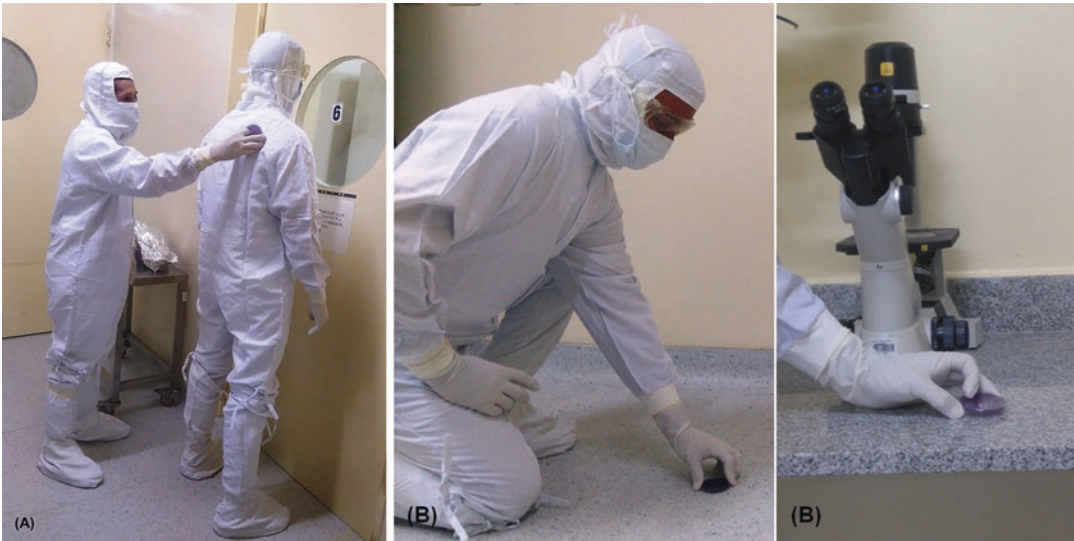
Fig. 19 Verifications of (a) sterile gowning; (b) efficacy of laboratory-surface disinfection by Quality Assurance
