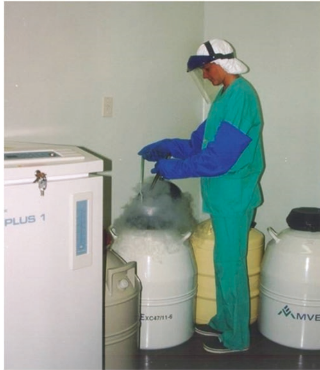
Fig. 11 Extraction of frozen cell ampoules from liquid nitrogen for thawing and establishing new cultures
