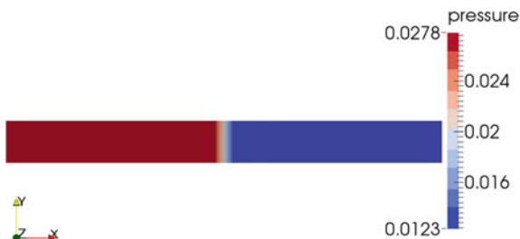
Fig. 10.10 Pressure distribution of the sealed test (case 1)
