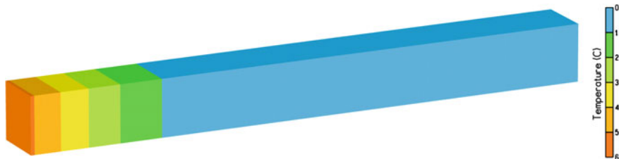
Fig. 10.5 Temperature distribution after 10,000 s
