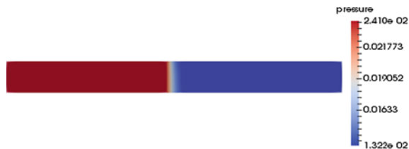
Fig. 10.14 Pressure distribution in the composite beam
