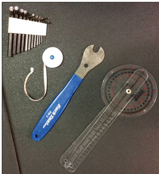
Fig. 16.3 Basic equipment necessary to perform a basic bike fit assessment [allen wrenches (ideally also a torque wrench), tape measure (also used as a make-shift plumb bob), pedal wrench, and goniometer] (bike trainer not shown)
