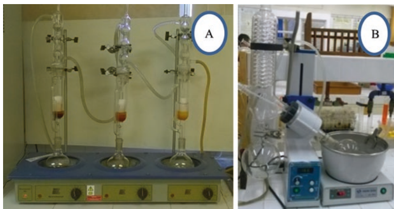
Fig. 1.33 Determination of extractables. (a) Successive extraction in soxhlet equipment, (b) separation of extractables in rotary evaporator
