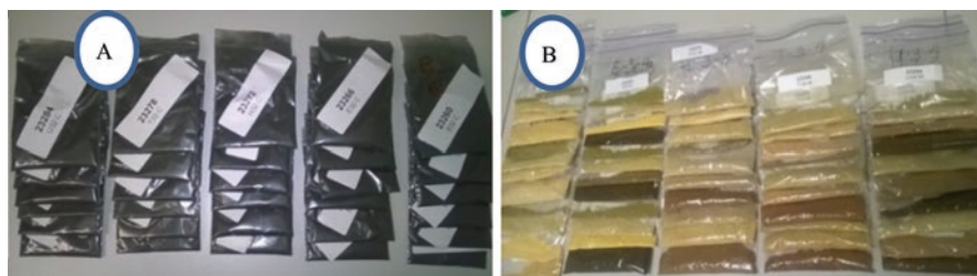
Fig. 1.25 Samples of size 425 \mu\text{m} : (a) charcoal of trunk and branches, (b) flour of trunks, branches, twigs, and leaves of the five studied species
