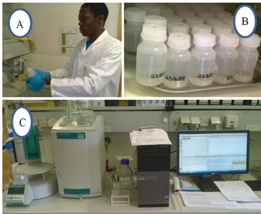
Fig. 1.37 Analysis of post-combustion residue: (a) recovery and dilution of the residues, (b) cooling of diluted solutions, (c) ionic chromatography and data record
