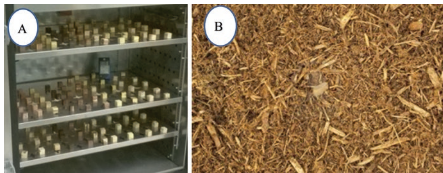
Fig. 1.22 Preparation of samples: (a) conditioning of test pieces in the chamber, (b) drying of chips in air
