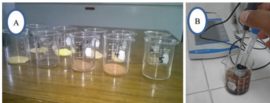
Fig. 1.35 Determination of pH: (a) samples in beakers, (b) reading in potentiometer
