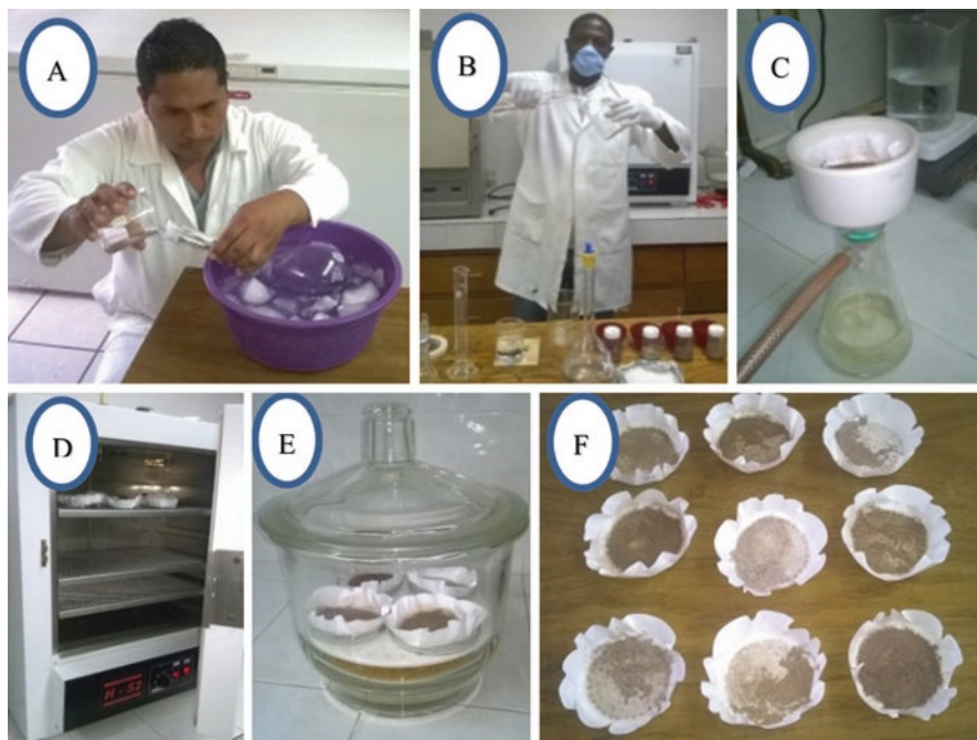
Fig. 1.34 Determination of lignin content: (a) preparation of solutions \text{H}_2\text{SO}_4 and \text{HBr} , (b) addition of acids to the flour sample, (c) extractable filtering and washing of acid residues, (d) drying in furnace, (e) desiccator with lignin samples, (f) lignin
