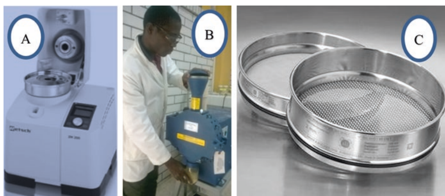
Fig. 1.24 Preparation of samples through (a) milling of charcoal, (b) milling of chips and dry leaves, (c) sieves of 40 and 60 holes
