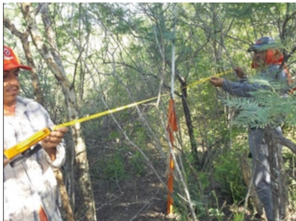
Fig. 1.16 Measurement of the projection of canopy coverage of tree and shrubs
