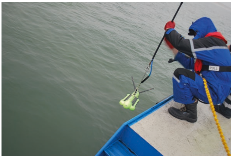
Fig. 2.14 Launching of the Klein 3900 side scan sonar (Photo by Algridas Stankevičius)
