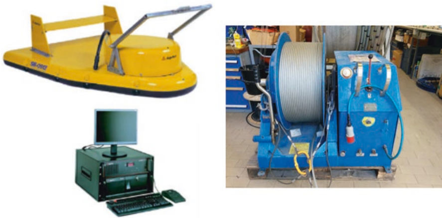
Fig. 2.24 Edge Tech SB216S towfish, deck unit, and deck winch
