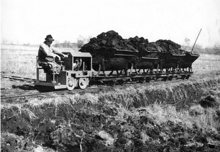
Fig. 2.6 Transport of peat material with a diesel locomotive to the specialist clinic Teufelsbad in Blankenburg, Germany (Pawel et al. 2013, p. 37; Photo: Fundus Teufelsbad, with kind permission from Bergverein zu Hüttenrode e. V.)
