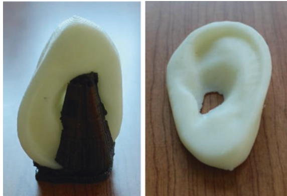
Fig. 2 Physical part with its support material before and after the removal process
