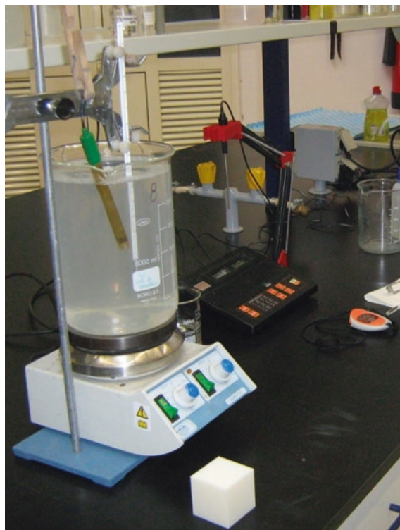
Fig. 8 Experimental setup for the dissolution of the support material blocks
