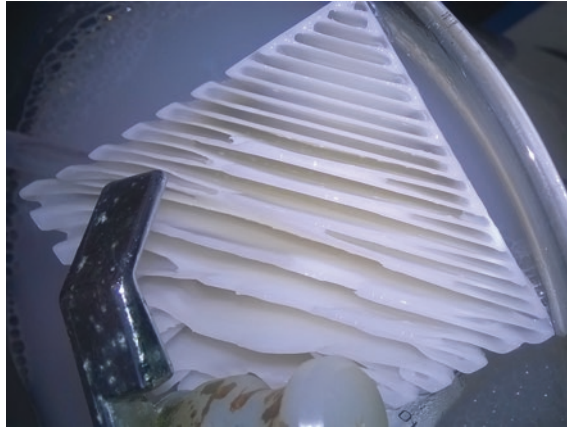
Fig. 9 Illustration of the dissolution process of one of the support material blocks
