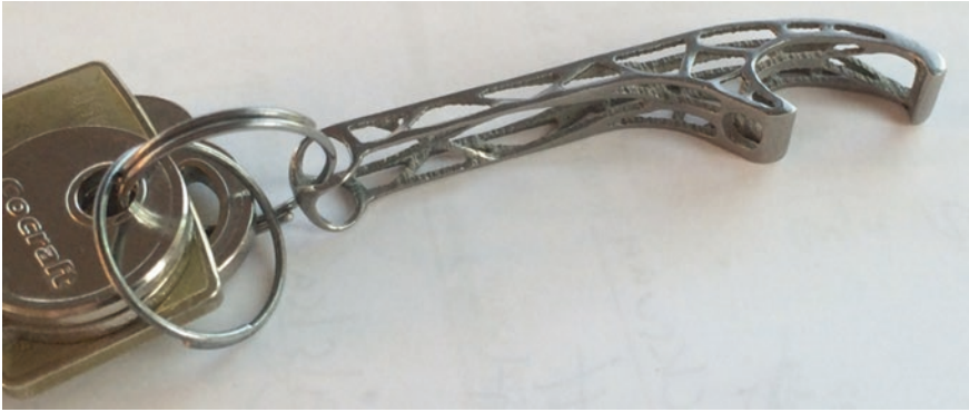
Fig. 2 Additively manufactured titanium bottle opener in which a 90 % material saving was made compared to a bottle-opener made though CNC machining, as conventional manufacturing would be unable to achieve the internal complexity of the component. It was produced in titanium 64 on a selective laser melting system using topology optimization to remove as much material as possible while maintaining the required mechanical characteristics (Diegel 2015)
