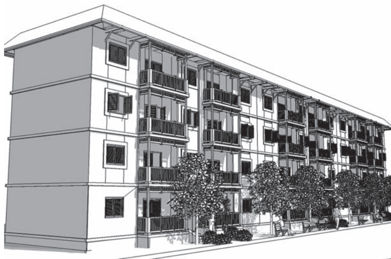
FIGURE 7.4. El Vallecito, a public housing complex in Guanahacabibes Peninsula, extreme western Pinar del Río Province, 2007. Shown here is the GP-4 ( Gran Panel ) design commonly used during the socialist period. Thousands of units were built across the island. The photograph (top) shows clotheslines, few trees, solid concrete balconies, and even tobacco leaf drying (upper left balconies). Computer-aided design (CAD) proposal (bottom) remedies some of these issues (e.g., visual clutter), but mainly provides more shade and improves air circulation by using trees and new eaves and balconies. Wood and stone materials come from the local area. Photograph and CAD courtesy Mabel Matamoros Tuma.
