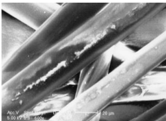
Fig. 21 SEM image of cold plasma-treated milkweed fibre showing surface corrosion (Reproduced with permission from [63])
