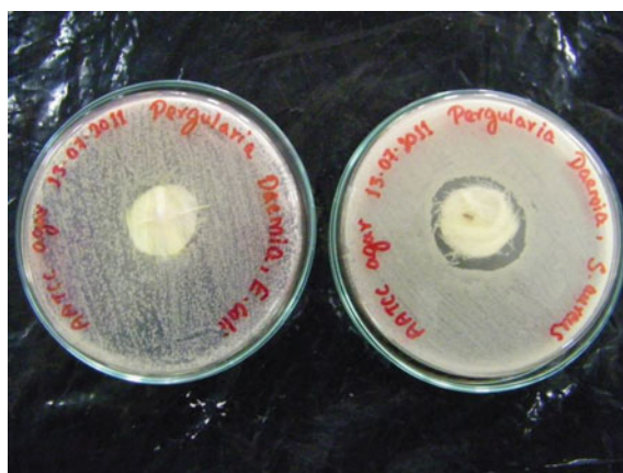
Fig. 14 Antibacterial activity of raw milkweed fibre against Staphylococcus aureus and Escherichia coli
