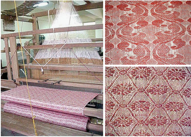
Fig. 2 Full view of the handloom developed with a Jacquard-shedding arrangement for diverse product and ornamental fabric development [24]
