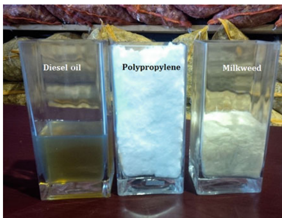
Fig. 22 Oil sorption capacity of polypropylene and milkweed fibres (Reproduced with permission from [83])
