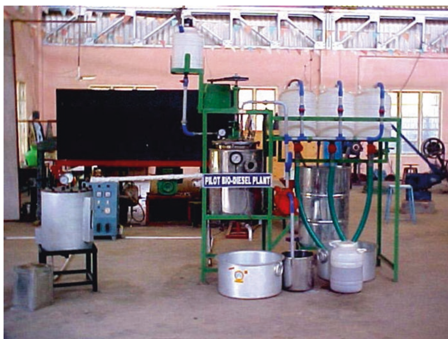
Fig. 3 Biodiesel pilot plant (College & Research Institute Tamil Nadu Agricultural University, India)
