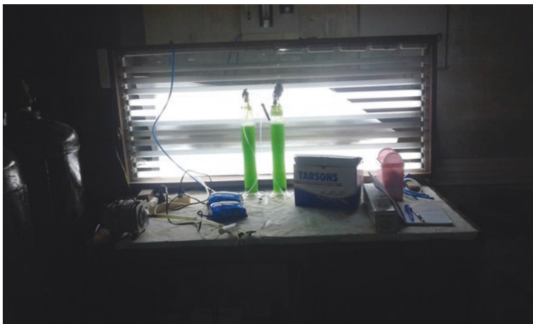
Fig. 2 Experimental setup for studying growth kinetics of algae using polythene combustion gas
