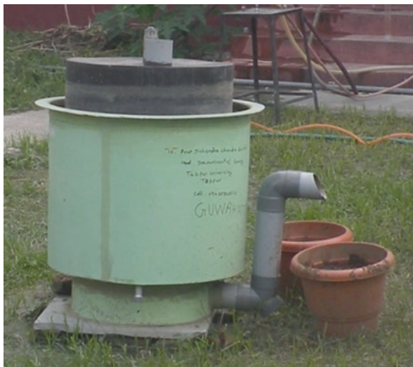
Fig. 1 Anaerobic digester unit with digestate collection outlet
