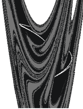
Fig. 21.18. Three basins of attraction for the Hénon map x_{n+1} = ay_n + 1 - x_n^2 , y_{n+1} = bx_n , with a = 0.475 .
